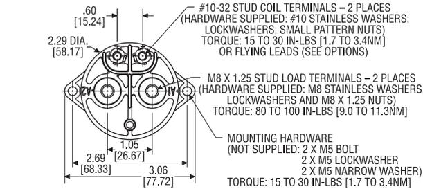
**Note:** When stud terminals are specified for coil connections, the electrical connection is made at the tab located at the base of the stud.
