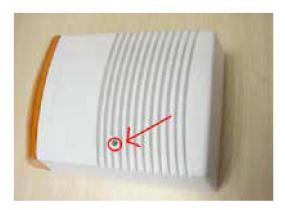
2. Open the housing. Place 3x AA 1.5 V batteries in the battery compartment, matching the polarity markings (+ and -) to activate the flashing LED. Close the housing and replace the screw after placing the batteries.
