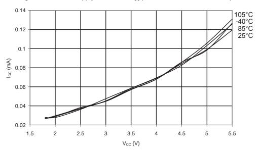
Figure 31-240. ATmega168PA: Active Supply Current vs. V<sub>CC</sub> (Internal RC Oscillator, 1MHz)
