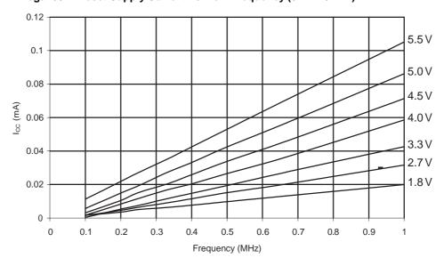
Figure 31-235. ATmega168A: Reset Supply Current vs. Frequency (1 - 20MHz)
