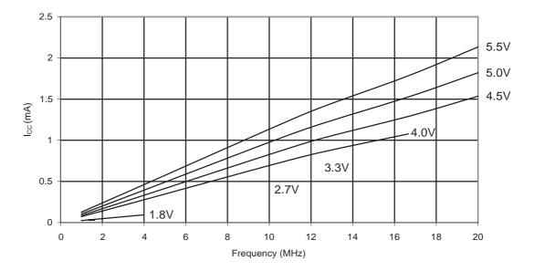
Figure 33-8. ATmega88PA: Idle Supply Current vs. V<sub>CC</sub> (Internal RC Oscillator, 128kHz)
