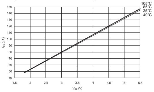
Figure 32-41.ATmega48PA: Brownout Detector Current vs. V<sub>CC</sub>
