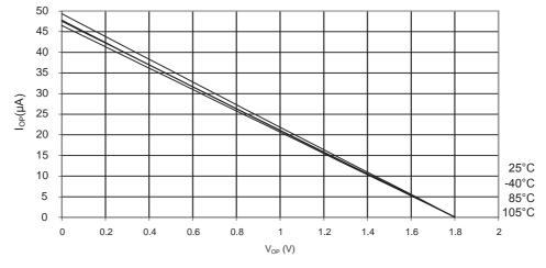
Figure 35-16.ATmega328P: I/O Pin Pull-up Resistor Current vs. Input Voltage (V<sub>CC</sub> = 2.7V)
