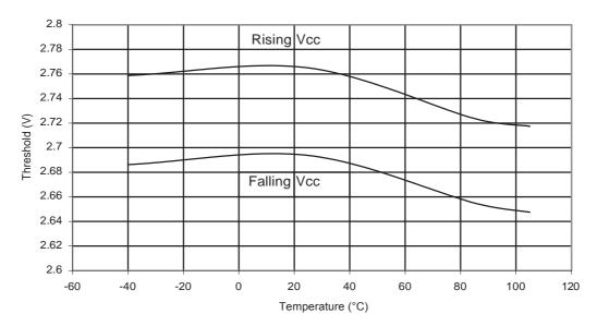
Figure 33-32.ATmega88PA: BOD Thresholds vs. Temperature (BODLEVEL is 4.3V)
