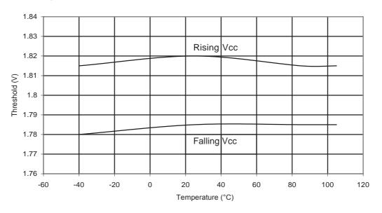
Figure 33-31.ATmega88PA: BOD Thresholds vs. Temperature (BODLEVEL is 2.7V)
