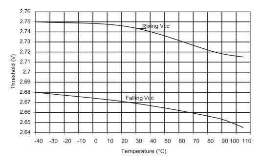
Figure 32-32.ATmega48PA: BOD Thresholds vs. Temperature (BODLEVEL is 4.3V)
