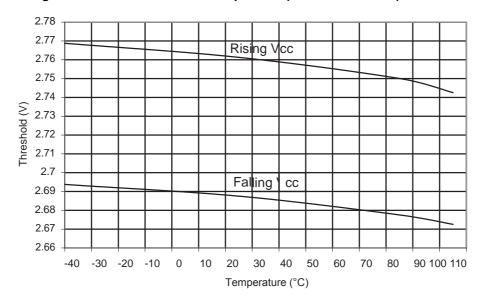
Figure 35-33.ATmega328P: BOD Thresholds vs. Temperature (BODLEVEL is 4.3V)
