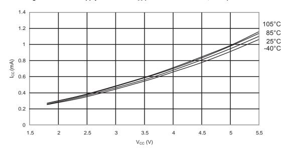
Figure 33-5. ATmega88PA: Active Supply Current vs. V<sub>CC</sub> (Internal RC Oscillator, 8MHz)
