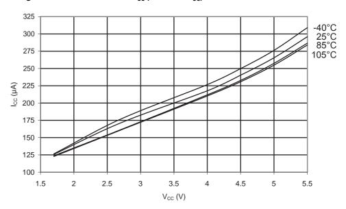
Figure 34-42.ATmega168PA: Analog Comparator Current vs. V<sub>CC</sub>
