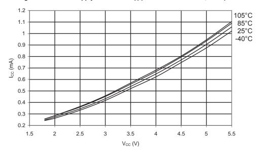
Figure 31-241. ATmega168PA: Active Supply Current vs. V<sub>CC</sub> (Internal RC Oscillator, 8MHz)
