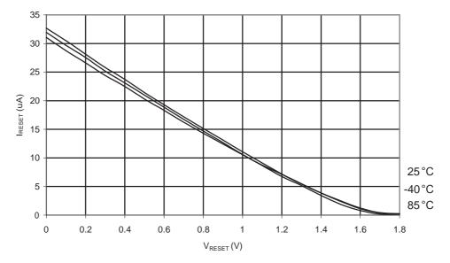
Figure 31-19. ATmega48A: Reset Pull-up Resistor Current vs. Reset Pin Voltage (V<sub>CC</sub> = 2.7 V)
