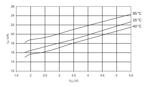
Figure 31-233. ATmega168A: Programming Current vs. V<sub>CC</sub>
