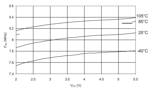
Figure 35-38.ATmega328P: Calibrated 8MHz RC Oscillator Frequency vs. Temperature
