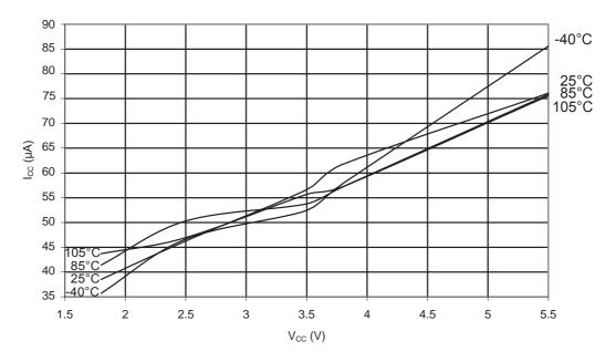
Figure 31-89. ATmega48PA: AREF External Reference Current vs.  $V_{\text{CC}}$
