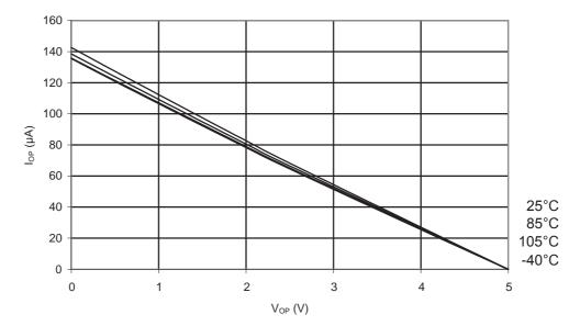
Figure 35-18.ATmega328P: Reset Pull-up Resistor Current vs. Reset Pin Voltage (V<sub>CC</sub> = 1.8V)
