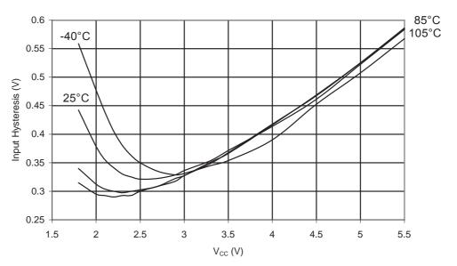
Figure 34-28.ATmega168PA: Reset Input Threshold Voltage vs. V<sub>CC</sub> (V<sub>IH</sub>, I/O Pin read as '1')
