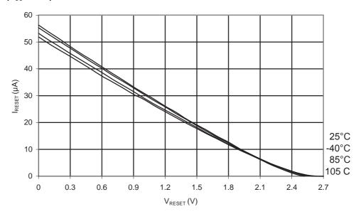
Figure 31-256. ATmega168PA: Reset Pull-up Resistor Current vs. Reset Pin Voltage (V<sub>CC</sub> = 5V)
