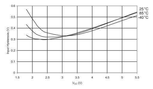
Figure 31-28. ATmega48A: Reset Input Threshold Voltage vs. V<sub>CC</sub> (V<sub>III</sub>, I/O Pin read as '1)'
