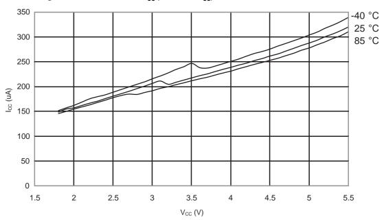
Figure 31-325. ATmega328: Analog Comparator Current vs. V<sub>CC</sub>
