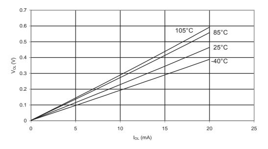
Figure 31-164. ATmega88PA: I/O Pin Output Voltage vs. Source Current (Vcc = 3V)
