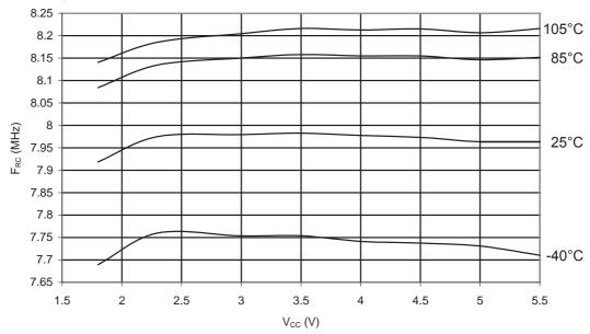
Figure 32-36.ATmega48PA: Calibrated 8MHz RC Oscillator Frequency vs. Temperature
