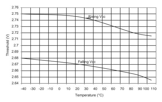
Figure 31-80. ATmega48PA: BOD Thresholds vs. Temperature (BODLEVEL is 4.3V)
