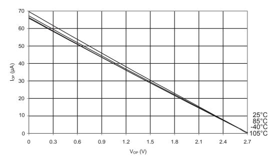
Figure 31-64. ATmega48PA: I/O Pin Pull-up Resistor Current vs. Input Voltage (V<sub>CC</sub> = 5V)
