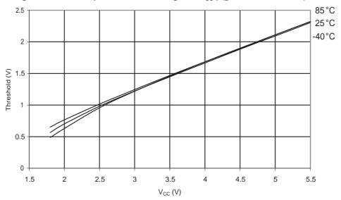
Figure 31-216. ATmega168A: I/O Pin Input Hysteresis vs. V<sub>CC</sub>
