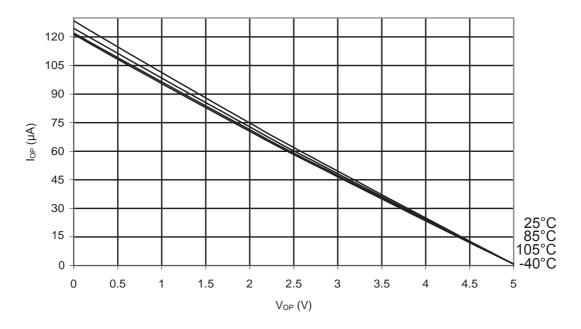
Figure 31-65. ATmega48PA: Reset Pull-up Resistor Current vs. Reset Pin Voltage (V<sub>CC</sub> = 1.8V)
