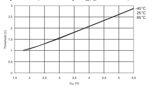
Figure 31-26. ATmega48A: I/O Pin Input Threshold Voltage vs. V<sub>CC</sub> (V<sub>IL</sub>, I/O Pin read as '0')
