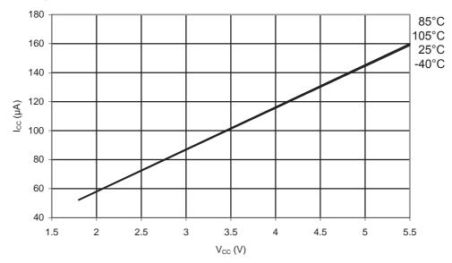
Figure 31-374. ATmega328P: Brownout Detector Current vs. V<sub>CC</sub>
