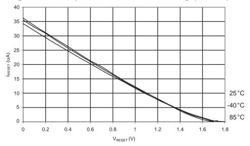
Figure 31-113. ATmega88A: Reset Pull-up Resistor Current vs. Reset Pin Voltage (V<sub>CC</sub> = 2.7 V)
