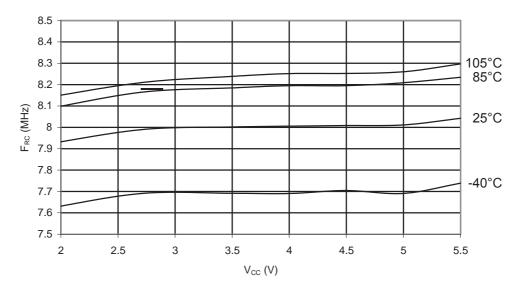
Figure 34-39.ATmega168PA: Calibrated 8MHz RC Oscillator Frequency vs. Temperature
