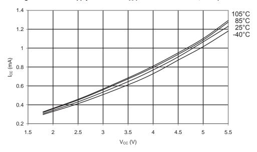
Figure 31-336. ATmega328P: Active Supply Current vs. V<sub>CC</sub> (Internal RC Oscillator, 8MHz)
