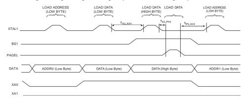
Note: 1. The timing requirements shown in Figure 29-6 (i.e.,  $t_{DVXH}$ ,  $t_{XHXL}$ , and  $t_{XLDX}$ ) also apply to loading operation.
