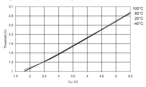
Figure 35-26.ATmega328P: I/O Pin Input Threshold Voltage vs.  $V_{CC}$  ( $V_{IL}$ , I/O Pin read as '0'
