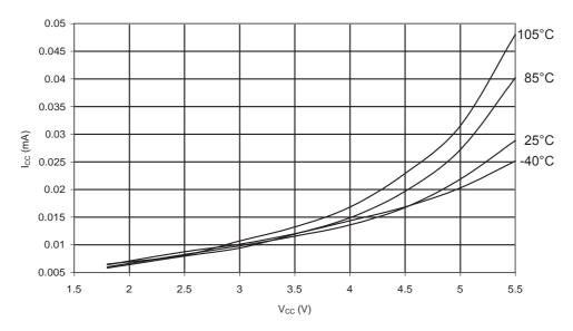
Figure 31-51. ATmega48PA: Active Supply Current vs. V<sub>CC</sub> (Internal RC Oscillator, 1MHz)
