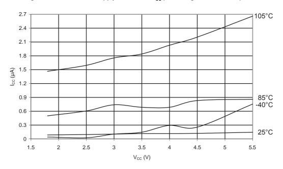
Figure 32-12.ATmega48PA: Power-Down Supply Current vs. V<sub>CC</sub> (Watchdog Timer Enabled)
