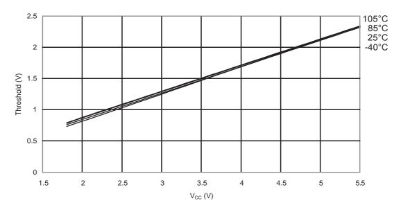
Figure 31-171. ATmega88PA: Reset Pin Input Hysteresis vs. V<sub>CC</sub>
