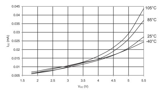
Figure 34-9. ATmega168PA: Idle Supply Current vs. V<sub>CC</sub> (Internal RC Oscillator, 1MHz)
