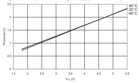
Figure 31-30. ATmega48A: Reset Pin Input Hysteresis vs.  $V_{CC}$
