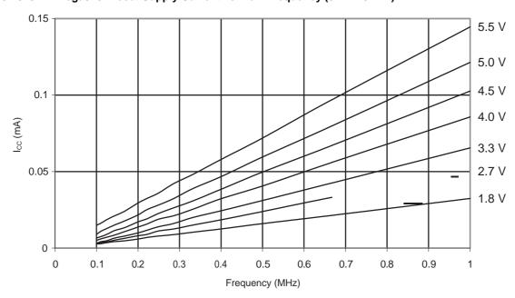
Figure 31-330. ATmega328: Reset Supply Current vs. Frequency (1 - 20MHz)
