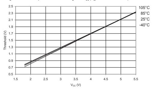
Figure 35-30.ATmega328P: Reset Pin Input Hysteresis vs. V<sub>CC</sub>
