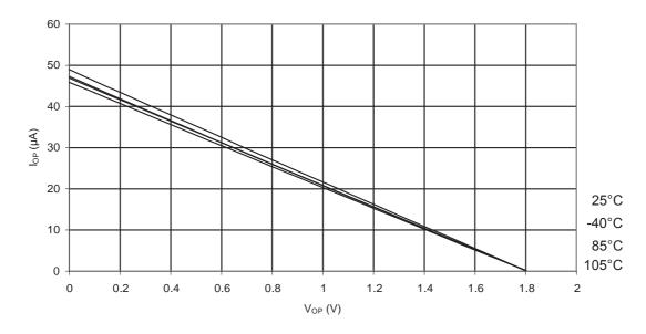
Figure 31-157. ATmega88PA: I/O Pin Pull-up Resistor Current vs. Input Voltage (V<sub>CC</sub> = 2.7V)
