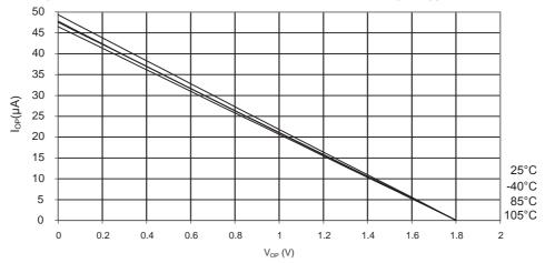
Figure 31-347. ATmega328P: I/O Pin Pull-up Resistor Current vs. Input Voltage (V<sub>CC</sub> = 2.7V)
