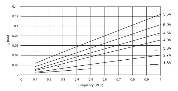
Figure 31-143. ATmega88PA: Active Supply Current vs. Frequency (1 - 20MHz)
