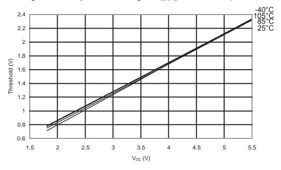
Figure 31-77. ATmega48PA: Reset Pin Input Hysteresis vs. V<sub>CC</sub>
