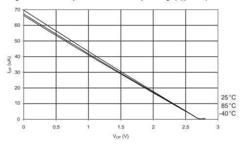
Figure 31-17. ATmega48A: I/O Pin Pull-up Resistor Current vs. Input Voltage (V<sub>CC</sub> = 5V)
