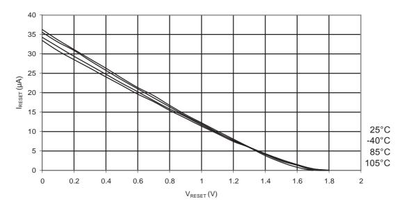
Figure 31-160. ATmega88PA: Reset Pull-up Resistor Current vs. Reset Pin Voltage (V<sub>CC</sub> = 2.7V)
