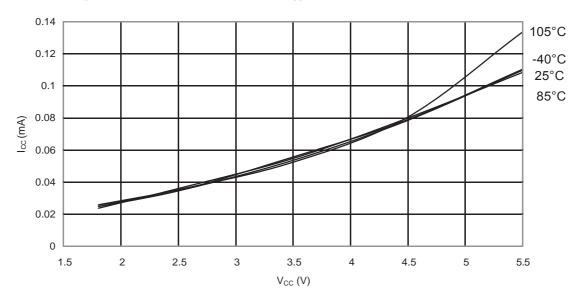
Figure 31-145. ATmega88PA: Active Supply Current vs. V<sub>CC</sub> (Internal RC Oscillator, 1MHz)
