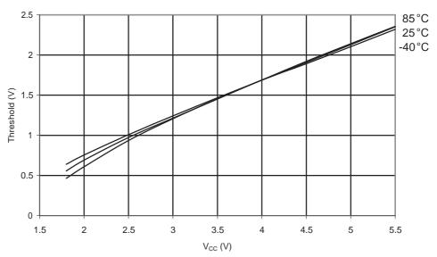
Figure 31-27. ATmega48A: I/O Pin Input Hysteresis vs. V<sub>CC</sub>
