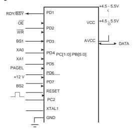
Note:  $V_{CC}$  - 0.3V < AV<sub>CC</sub> <  $V_{CC}$  + 0.3V, however, AV<sub>CC</sub> should always be within 4.5 - 5.5V
