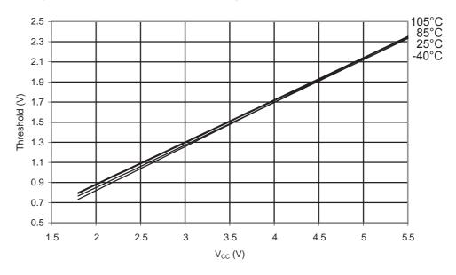
Figure 31-266. ATmega168PA: Reset Pin Input Hysteresis vs. V<sub>CC</sub>
