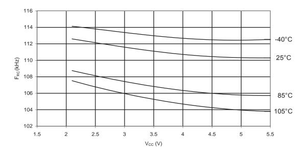
Figure 31-179. ATmega88PA: Calibrated 8MHz RC Oscillator Frequency vs. V<sub>CC</sub>
