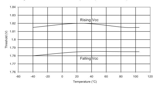
Figure 31-173. ATmega88PA: BOD Thresholds vs. Temperature (BODLEVEL is 2.7V)
