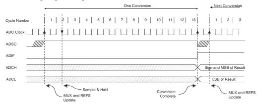
Figure 24-6. ADC Timing Diagram, Auto Triggered Conversion
