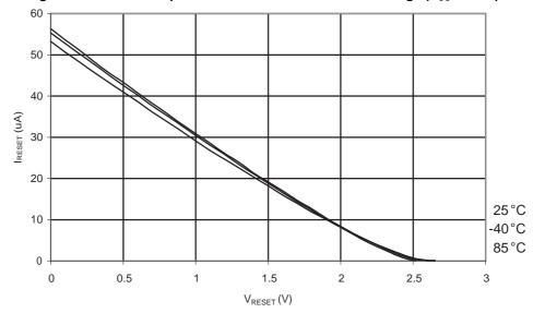
Figure 31-209. ATmega168A: Reset Pull-up Resistor Current vs. Reset Pin Voltage (V<sub>CC</sub> = 5V)
