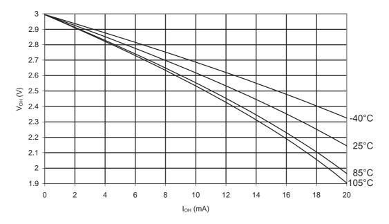
Figure 32-23.ATmega48PA: I/O Pin Output Voltage vs. Source Current (V<sub>CC</sub> = 5V)
