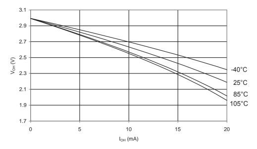
Figure 34-24.ATmega168PA: I/O Pin Output Voltage vs. Source Current (V<sub>CC</sub> = 5V)
