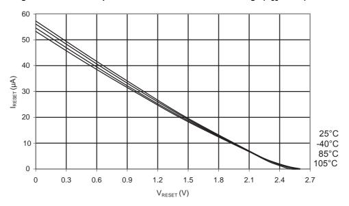
Figure 35-20.ATmega328P: Reset Pull-up Resistor Current vs. Reset Pin Voltage (V<sub>CC</sub> = 5V)
