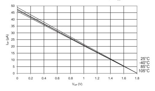
Figure 34-16.ATmega168PA: I/O Pin Pull-up Resistor Current vs. Input Voltage (V<sub>CC</sub> = 2.7V)
