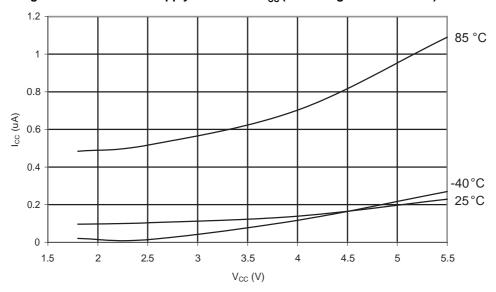
Figure 31-12. ATmega48A: Power-Down Supply Current vs. V<sub>CC</sub> (Watchdog Timer Enabled)
