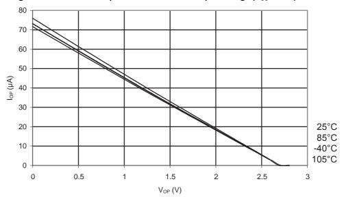
Figure 34-17.ATmega168PA: I/O Pin Pull-up Resistor Current vs. Input Voltage (V<sub>CC</sub> = 5V)
