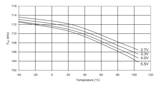
Figure 33-34.ATmega88PA: Watchdog Oscillator Frequency vs. V<sub>CC</sub>
