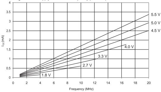
Figure 31-292. ATmega328: Idle Supply Current vs. V<sub>CC</sub> (Internal RC Oscillator, 128kHz)
