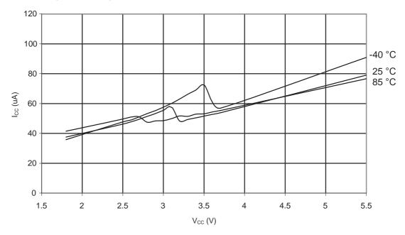
Figure 31-326. ATmega328: AREF External Reference Current vs. V<sub>CC</sub>
