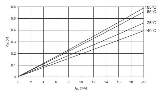
Figure 31-259. ATmega168PA: I/O Pin Output Voltage vs. Source Current (V<sub>CC</sub> = 3V)
