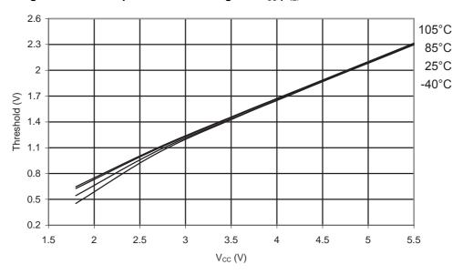
Figure 35-27.ATmega328P: I/O Pin Input Hysteresis vs.  $V_{\rm CC}$
