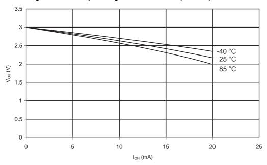
Figure 31-308. ATmega328: I/O Pin Output Voltage vs. Source Current (V<sub>CC</sub> = 5 V)
