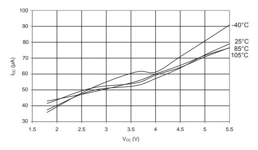
Figure 31-373. ATmega328P: AREF External Reference Current vs. V<sub>CC</sub>
