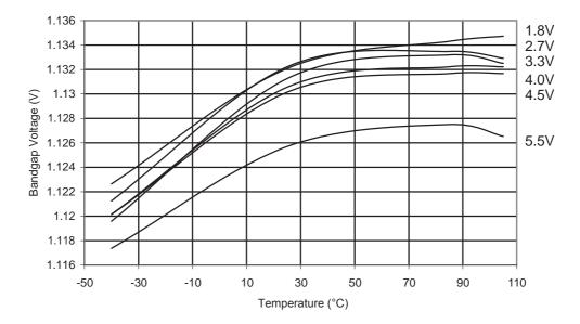
Figure 31-271. ATmega168PA: Calibrated Bandgap Voltage vs. Vcc
