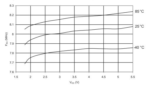
Figure 31-132. ATmega88A: Calibrated 8MHz RC Oscillator Frequency vs. Temperature
