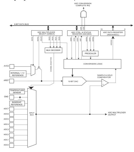
Figure 24-1. Analog to Digital Converter Block Schematic Operation
