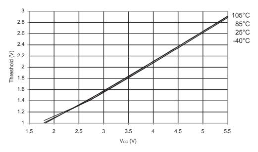
Figure 31-262. ATmega168PA: I/O Pin Input Threshold Voltage vs. V<sub>CC</sub> (V<sub>IL</sub>, I/O Pin read as '0')
