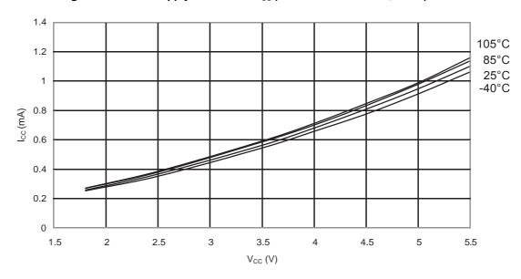
Figure 31-146. ATmega88PA: Active Supply Current vs. V<sub>CC</sub> (Internal RC Oscillator, 8MHz)
