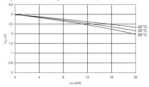
Figure 31-24. ATmega48A: I/O Pin Output Voltage vs. Source Current (V<sub>CC</sub> = 5 V)
