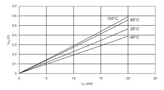
Figure 33-22.ATmega88PA: I/O Pin Output Voltage vs. Source Current (Vcc = 3V)
