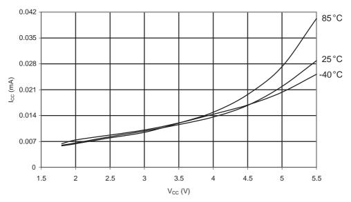
Figure 31-9. ATmega48A: Idle Supply Current vs. V<sub>CC</sub> (Internal RC Oscillator, 1MHz)
