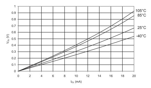
Figure 34-22.ATmega168PA: I/O Pin Output Voltage vs. Sink Current (V<sub>CC</sub> = 5V)
