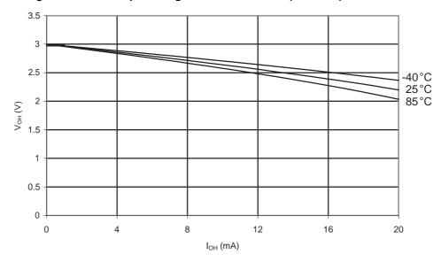
Figure 31-118. )ATmega88A: I/O Pin Output Voltage vs. Source Current ( $V_{CC} = 5 \text{ V}$ )
