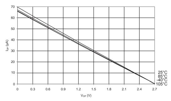
Figure 32-16.ATmega48PA: I/O Pin Pull-up Resistor Current vs. Input Voltage (V<sub>CC</sub> = 5V)
