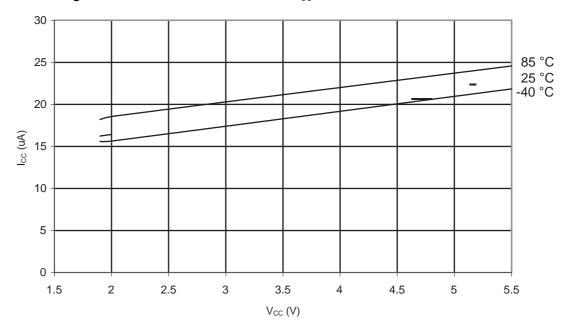
Figure 31-328. ATmega328: Programming Current vs. V<sub>CC</sub>
