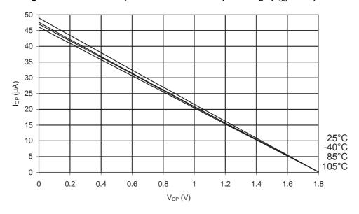
Figure 31-252. ATmega168PA: I/O Pin Pull-up Resistor Current vs. Input Voltage (V<sub>CC</sub> = 2.7V)
