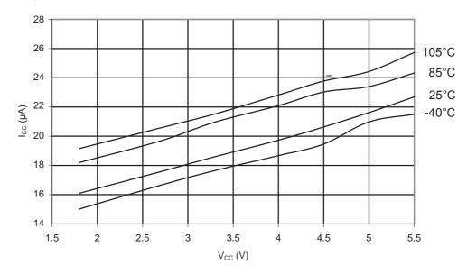
Figure 34-45.ATmega168PA: Programming Current vs. V<sub>CC</sub>
