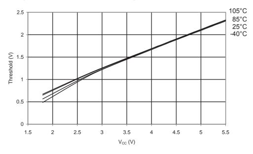
Figure 31-263. ATmega168PA: I/O Pin Input Hysteresis vs. V<sub>CC</sub>
