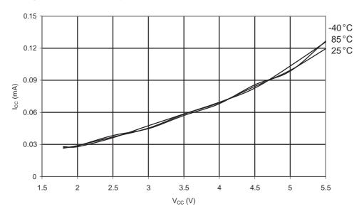
Figure 31-193. ATmega168A: Active Supply Current vs. V<sub>CC</sub> (Internal RC Oscillator, 1MHz)
