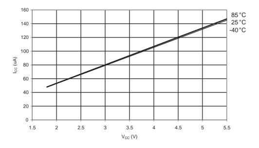
Figure 31-43. ATmega48A Brownout Detector Current vs. V<sub>CC</sub>
