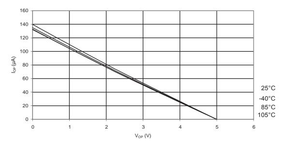
Figure 33-17.ATmega88PA: Reset Pull-up Resistor Current vs. Reset Pin Voltage (V<sub>CC</sub> = 1.8V)
