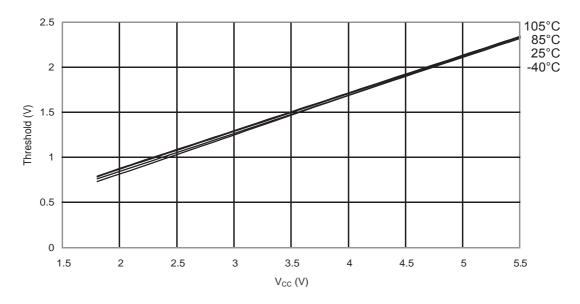
Figure 33-29.ATmega88PA: Reset Pin Input Hysteresis vs. V<sub>CC</sub>
