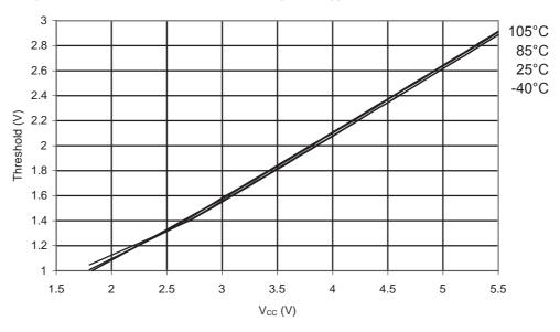
Figure 34-26.ATmega168PA: I/O Pin Input Threshold Voltage vs. V<sub>CC</sub> (V<sub>IL</sub>, I/O Pin read as '0')
