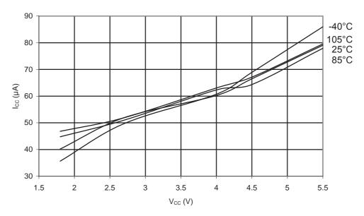
Figure 31-279. ATmega168PA: AREF External Reference Current vs. V<sub>CC</sub>
