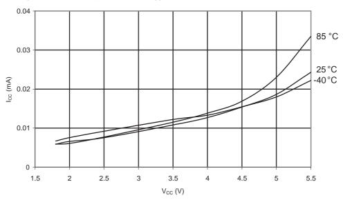
Figure 31-103. ATmega88A: Idle Supply Current vs. V<sub>CC</sub> (Internal RC Oscillator, 1MHz)
