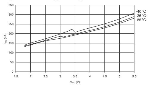
Figure 31-41. ATmega48A: Analog Comparator Current vs. V<sub>CC</sub>
