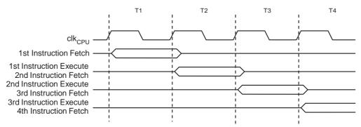
Figure 7-5 shows the internal timing concept for the Register File. In a single clock cycle an ALU operation using two register operands is executed, and the result is stored back to the destination register.
