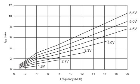
Figure 31-3. ATmega48A: Active Supply Current vs. V<sub>CC</sub> (Internal RC Oscillator, 128kHz)
