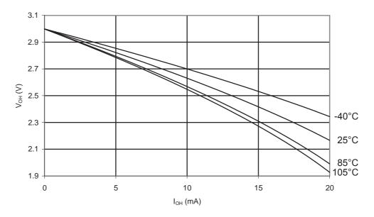
Figure 31-355. ATmega328P: I/O Pin Output Voltage vs. Source Current (V<sub>CC</sub> = 5V)
