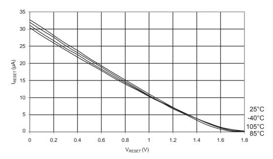
Figure 32-18.ATmega48PA: Reset Pull-up Resistor Current vs. Reset Pin Voltage (V<sub>CC</sub> = 2.7V)
