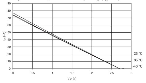
Figure 31-301. ATmega328: I/O Pin Pull-up Resistor Current vs. Input Voltage (V<sub>CC</sub> = 5 V)
