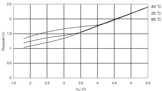
Figure 31-313. ATmega328: Reset Input Threshold Voltage vs. V<sub>CC</sub> (V<sub>IL</sub>, I/O Pin read as '0')
