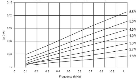
Figure 31-101. ATmega88A: Idle Supply Current vs. Frequency (1-20MHz)
