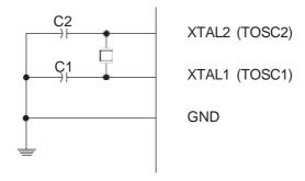
The Low Power Oscillator can operate in three different modes, each optimized for a specific frequency range. The operating mode is selected by the fuses CKSEL3...1 as shown in Table 9-3 on page 39.
