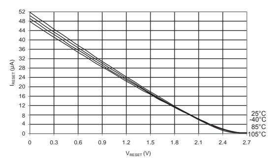
Figure 32-19.ATmega48PA: Reset Pull-up Resistor Current vs. Reset Pin Voltage (V<sub>CC</sub> = 5V)
