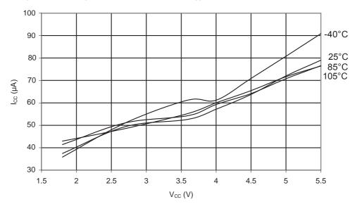
Figure 35-42.ATmega328P: AREF External Reference Current vs. V<sub>CC</sub>
