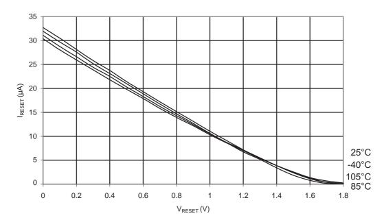
Figure 31-66. ATmega48PA: Reset Pull-up Resistor Current vs. Reset Pin Voltage (V<sub>CC</sub> = 2.7V)
