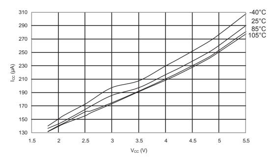
Figure 32-39.ATmega48PA: Analog Comparator Current vs.  $V_{\text{CC}}$
