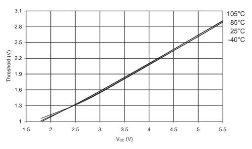
Figure 31-357. ATmega328P: I/O Pin Input Threshold Voltage vs.  $V_{CC}$  ( $V_{IL}$ , I/O Pin read as '0'
