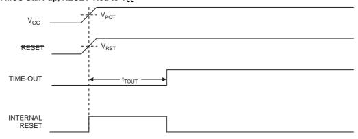
Figure 11-3. MCU Start-up, RESET Extended Externally
