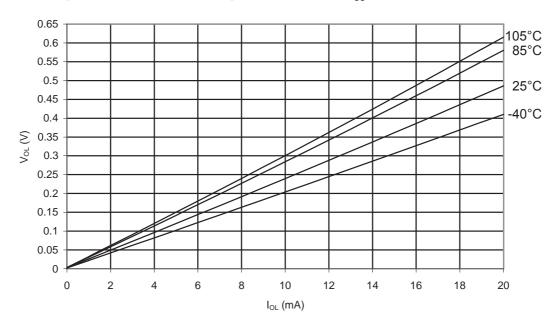
Figure 32-22.ATmega48PA: I/O Pin Output Voltage vs. Source Current (Vcc = 3V)
