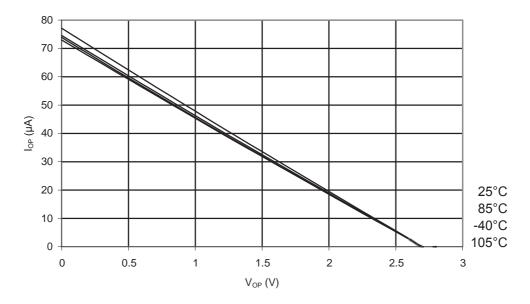
Figure 31-348. ATmega328P: I/O Pin Pull-up Resistor Current vs. Input Voltage (V<sub>CC</sub> = 5V)
