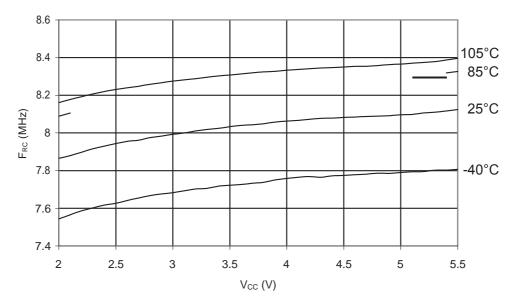
Figure 31-369. ATmega328P: Calibrated 8MHz RC Oscillator Frequency vs. Temperature
