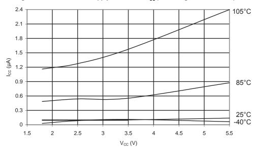
Figure 31-248. ATmega168PA: Power-Down Supply Current vs. V<sub>CC</sub> (Watchdog Timer Enabled)
