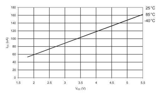
Figure 31-232. ATmega168A: Brownout Detector Current vs. V<sub>CC</sub>
