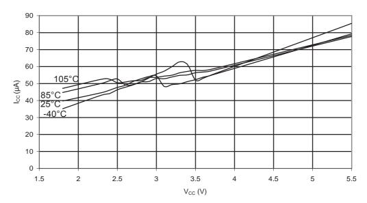
Figure 33-40.ATmega88PA: AREF External Reference Current vs. V<sub>CC</sub>
