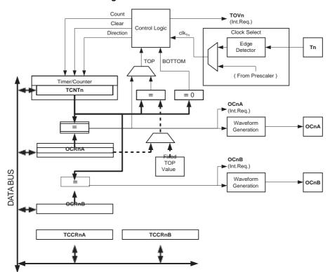
Figure 18-1. 8-bit Timer/Counter Block Diagram
