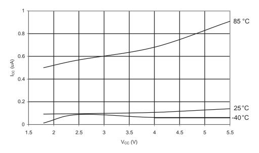
Figure 31-201. ATmega168A: Power-Down Supply Current vs. V<sub>CC</sub> (Watchdog Timer Enabled)
