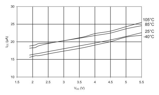
Figure 35-44.ATmega328P: Programming Current vs. V<sub>CC</sub>
