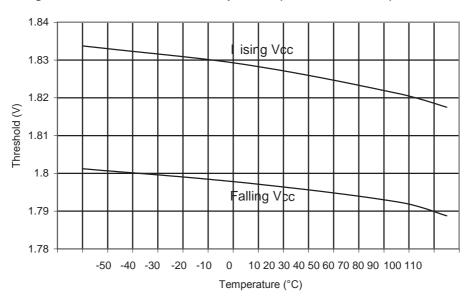
Figure 35-32.ATmega328P: BOD Thresholds vs. Temperature (BODLEVEL is 2.7V)
