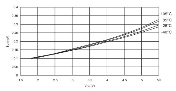
Figure 31-151. ATmega88PA: Idle Supply Current vs. V<sub>CC</sub> (Internal RC Oscillator, 8MHz)
