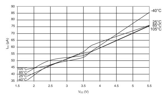
Figure 32-40.ATmega48PA: AREF External Reference Current vs. V<sub>CC</sub>
