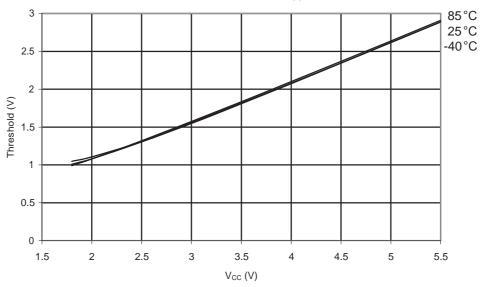
Figure 31-215. ATmega168A: I/O Pin Input Threshold Voltage vs.  $V_{CC}(V_{IL}, I/O Pin read as '0')$
