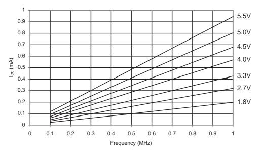
Figure 34-2. ATmega168PA: Active Supply Current vs. Frequency (1MHz - 20MHz)
