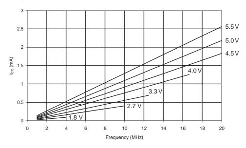
Figure 31-197. ATmega168A: Idle Supply Current vs. V<sub>CC</sub> (Internal RC Oscillator, 128kHz)
