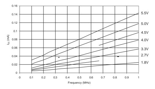
Figure 31-54. ATmega48PA: Idle Supply Current vs. Frequency (1-20MHz)
