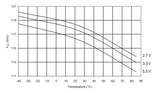
Figure 31-225. ATmega168A: Watchdog Oscillator Frequency vs. V<sub>CC</sub>
