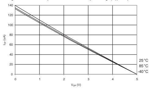
Figure 31-112. ATmega88A: Reset Pull-up Resistor Current vs. Reset Pin Voltage (V<sub>CC</sub> = 1.8 V)
