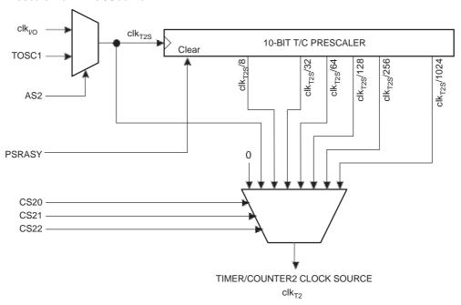
The clock source for Timer/Counter2 is named  $clk_{T2S}$ .  $clk_{T2S}$  is by default connected to the main system I/O clock  $clk_{IO}$ . By setting the AS2 bit in ASSR, Timer/Counter2 is asynchronously clocked from the TOSC1 pin. This enables use of Timer/Counter2 as a Real Time Counter (RTC). When AS2 is set, pins TOSC1 and TOSC2
