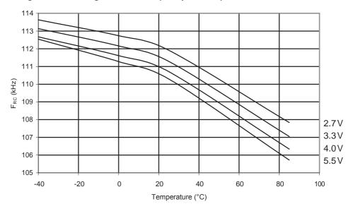
Figure 31-130. ATmega88A: Watchdog Oscillator Frequency vs. V<sub>CC</sub>
