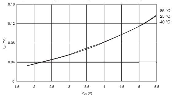
Figure 31-288. ATmega328: Active Supply Current vs. V<sub>CC</sub> (Internal RC Oscillator, 1MHz)
