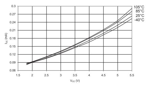
Figure 31-246. ATmega168PA: Idle Supply Current vs. V<sub>CC</sub> (Internal RC Oscillator, 8MHz)
