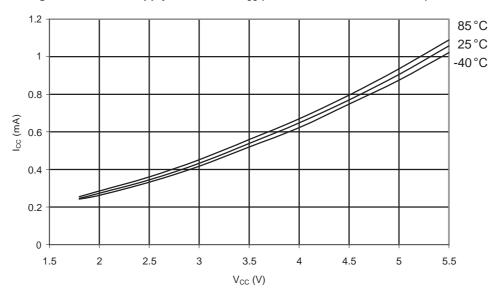
Figure 31-194. ATmega168A: Active Supply Current vs. V<sub>CC</sub> (Internal RC Oscillator, 8MHz)
