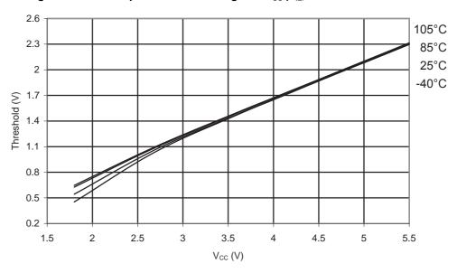
Figure 31-358. ATmega328P: I/O Pin Input Hysteresis vs.  $V_{\rm CC}$
