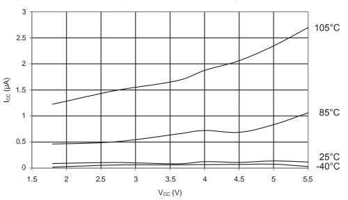
Figure 35-12.ATmega328P: Power-Down Supply Current vs. V<sub>CC</sub> (Watchdog Timer Enabled)
