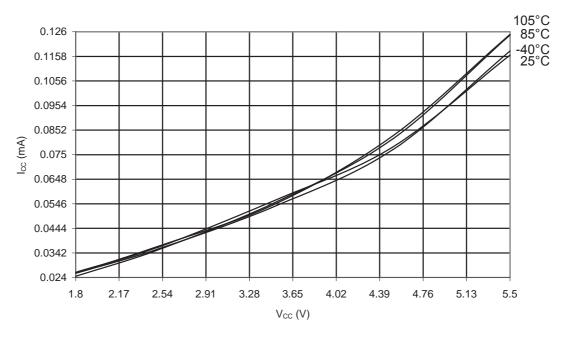
Figure 32-4. ATmega48PA: Active Supply Current vs. V<sub>CC</sub> (Internal RC Oscillator, 1MHz)
