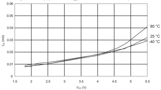
Figure 31-293. ATmega328: Idle Supply Current vs. V<sub>CC</sub> (Internal RC Oscillator, 1MHz)
