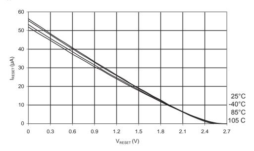
Figure 34-20.ATmega168PA: Reset Pull-up Resistor Current vs. Reset Pin Voltage (V<sub>CC</sub> = 5V)
