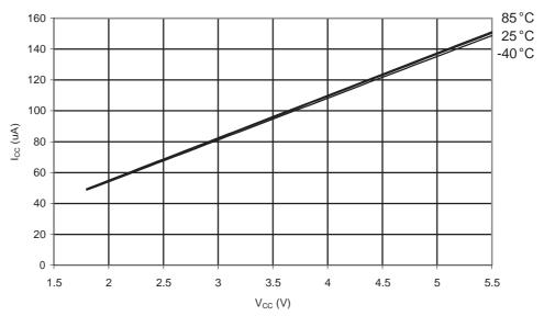
Figure 31-137. ATmega88A: Brownout Detector Current vs. V<sub>CC</sub>
