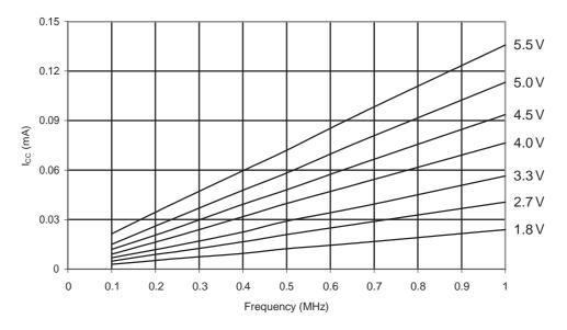
Figure 31-196. ATmega168A: Idle Supply Current vs. Frequency (1-20MHz)
