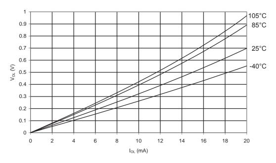
Figure 32-21.ATmega48PA: I/O Pin Output Voltage vs. Sink Current ( $V_{CC} = 5V$ )
