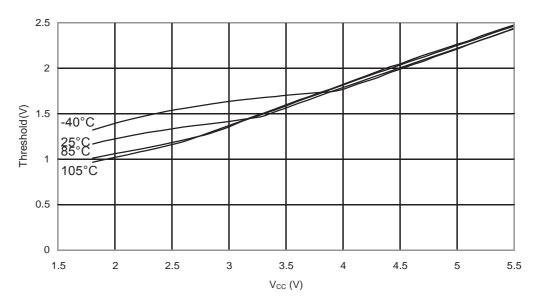
Figure 31-170. ATmega88PA: Reset Input Threshold Voltage vs. V<sub>CC</sub> (V<sub>IL</sub>, I/O Pin read as '0')
