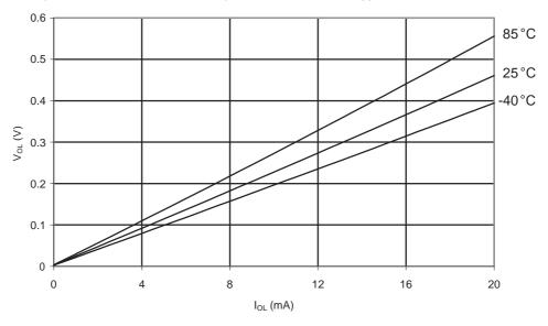
Figure 31-212. ATmega168A: I/O Pin Output Voltage vs. Source Current (Vcc = 3 V)
