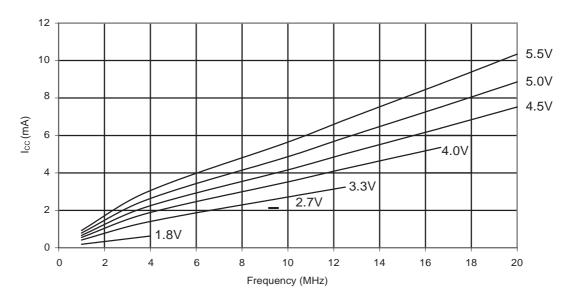
Figure 31-144. ATmega88PA: Active Supply Current vs. V<sub>CC</sub> (Internal RC Oscillator, 128kHz)
