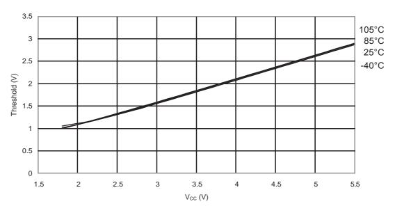
Figure 33-25.ATmega88PA: I/O Pin Input Threshold Voltage vs. V<sub>CC</sub> (V<sub>IL</sub>, I/O Pin read as '0')
