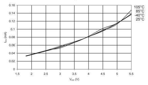
Figure 31-335. ATmega328P: Active Supply Current vs. V<sub>CC</sub> (Internal RC Oscillator, 1MHz)
