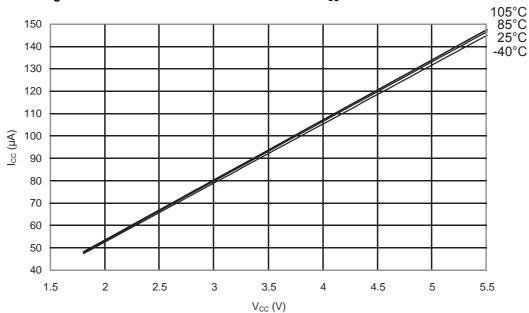
Figure 31-90. ATmega48PA: Brownout Detector Current vs. V<sub>CC</sub>
