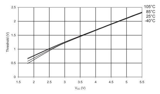
Figure 34-27.ATmega168PA: I/O Pin Input Hysteresis vs.  $V_{\rm CC}$
