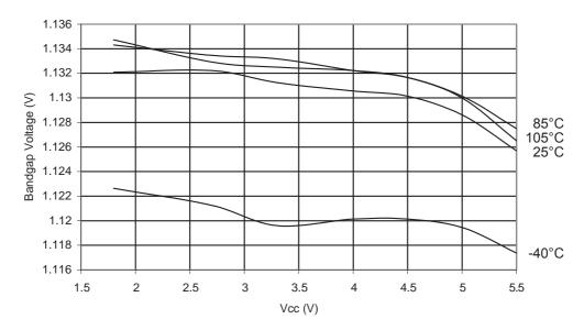
Figure 34-35.ATmega168PA: Calibrated Bandgap Voltage vs. Temperature
