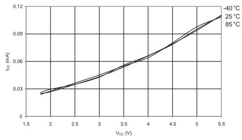
Figure 31-98. ATmega88A: Active Supply Current vs. V<sub>CC</sub> (Internal RC Oscillator, 1MHz)
