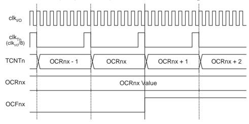
Figure 16-12 on page 139 shows the count sequence close to TOP in various modes. When using phase and frequency correct PWM mode the OCR1x Register is updated at BOTTOM. The timing diagrams will be the same, but TOP should be replaced by BOTTOM, TOP-1 by BOTTOM+1 and so on. The same renaming applies for modes that set the TOV1 Flag at BOTTOM.
