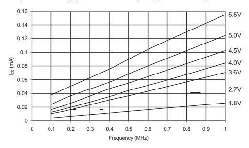
Figure 34-7. ATmega168PA: Idle Supply Current vs. Frequency (1MHz - 20MHz)
