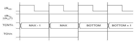
Figure 18-9 shows the same timing data, but with the prescaler enabled.
