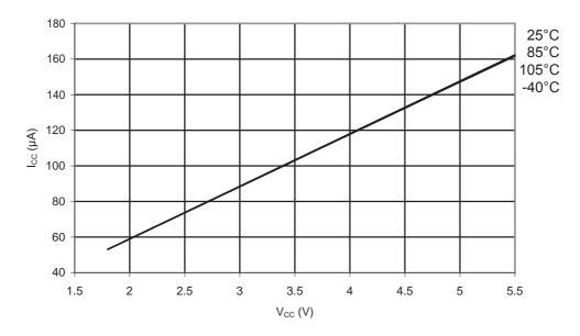
Figure 31-280. ATmega168PA: Brownout Detector Current vs. V<sub>CC</sub>
