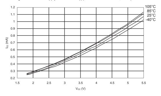
Figure 32-5. ATmega48PA: Active Supply Current vs. V<sub>CC</sub> (Internal RC Oscillator, 8MHz)
