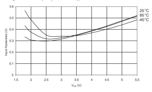
Figure 31-122. ATmega88A: Reset Input Threshold Voltage vs.  $V_{CC}(V_{Hr}, I/O Pin read as '1')$
