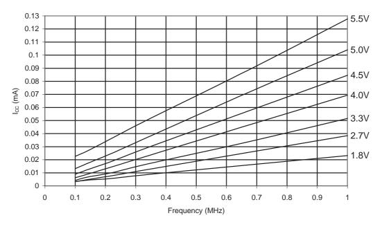
Figure 31-93. ATmega48PA: Reset Supply Current vs. Frequency (1MHz- 20MHz)
