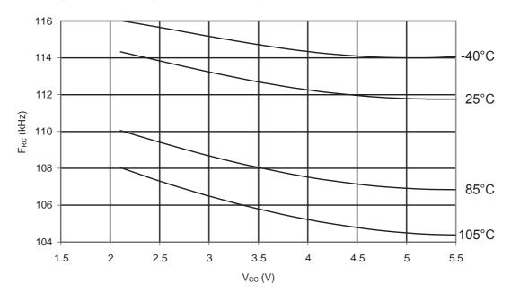
Figure 32-35.ATmega48PA: Calibrated 8MHz RC Oscillator Frequency vs. V<sub>CC</sub>
