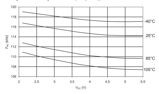
Figure 31-368. ATmega328P: Calibrated 8 MHz RC Oscillator Frequency vs.  $V_{\rm CC}$
