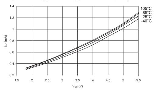
Figure 35-5. ATmega328P: Active Supply Current vs. V<sub>CC</sub> (Internal RC Oscillator, 8MHz)
