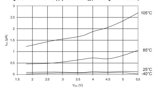
Figure 31-343. ATmega328P: Power-Down Supply Current vs. V<sub>CC</sub> (Watchdog Timer Enabled)
