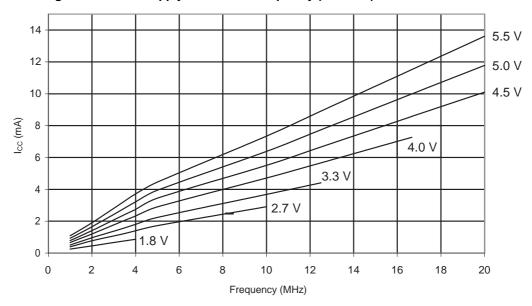
Figure 31-334. ATmega328P: Active Supply Current vs. V<sub>CC</sub> (Internal RC Oscillator, 128kHz)
