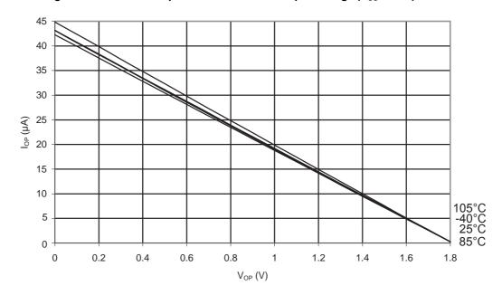
Figure 32-15.ATmega48PA: I/O Pin Pull-up Resistor Current vs. Input Voltage (V<sub>CC</sub> = 2.7V)
