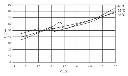
Figure 31-136. ATmega88A: AREF External Reference Current vs.  $V_{\text{CC}}$
