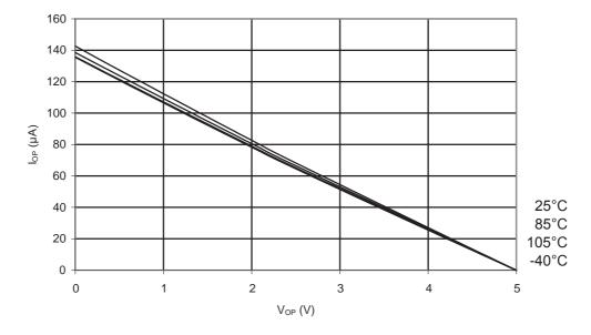
Figure 31-349. ATmega328P: Reset Pull-up Resistor Current vs. Reset Pin Voltage (V<sub>CC</sub> = 1.8V)
