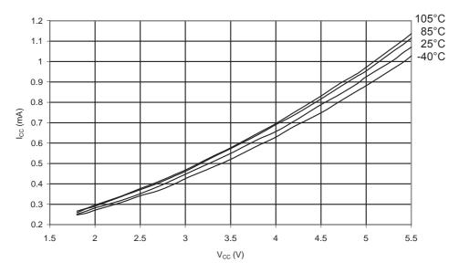
Figure 31-52. ATmega48PA: Active Supply Current vs. V<sub>CC</sub> (Internal RC Oscillator, 8MHz)
