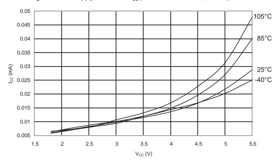
Figure 31-56. ATmega48PA: Idle Supply Current vs. V<sub>CC</sub> (Internal RC Oscillator, 1MHz)
