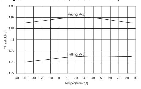
Figure 31-126. ATmega88A: BOD Thresholds vs. Temperature (BODLEVEL is 2.7 V)
