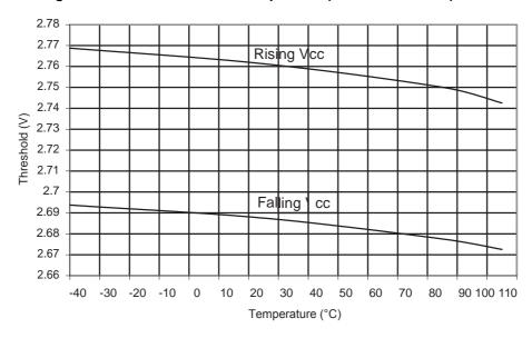
Figure 31-364. ATmega328P: BOD Thresholds vs. Temperature (BODLEVEL is 4.3V)
