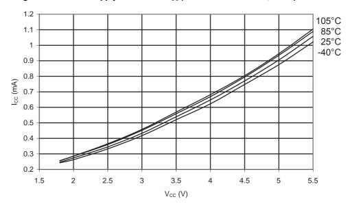
Figure 34-5. ATmega168PA: Active Supply Current vs. V<sub>CC</sub> (Internal RC Oscillator, 8MHz)
