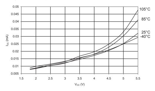
Figure 35-9. ATmega328P: Idle Supply Current vs. V<sub>CC</sub> (Internal RC Oscillator, 1MHz)
