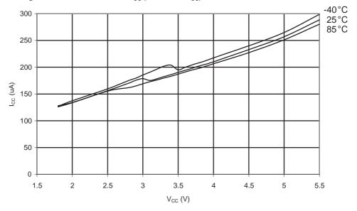
Figure 31-135. ATmega88A: Analog Comparator Current vs. V<sub>CC</sub>
