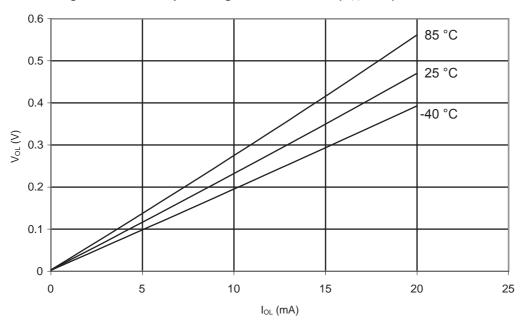
Figure 31-307. ATmega328: I/O Pin Output Voltage vs. Source Current (Vcc = 3 V)
