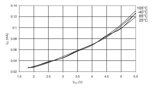
Figure 34-4. ATmega168PA: Active Supply Current vs. V<sub>CC</sub> (Internal RC Oscillator, 1MHz)
