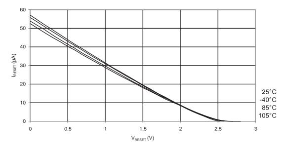
Figure 31-161. ATmega88PA: Reset Pull-up Resistor Current vs. Reset Pin Voltage (V<sub>CC</sub> = 5V)
