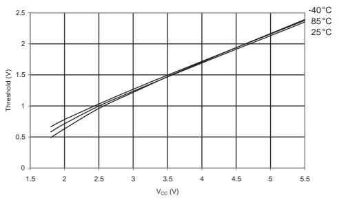
Figure 31-121. ATmega88A: I/O Pin Input Hysteresis vs. V<sub>CC</sub>
