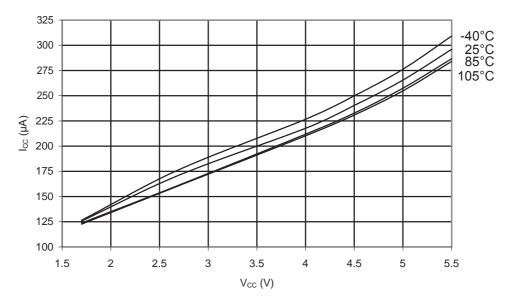
Figure 31-278. ATmega168PA: Analog Comparator Current vs. V<sub>CC</sub>
