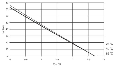
Figure 31-111. ATmega88A: I/O Pin Pull-up Resistor Current vs. Input Voltage (V<sub>CC</sub> = 5 V)
