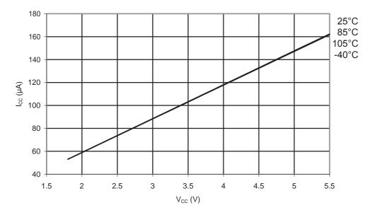
Figure 34-44.ATmega168PA: Brownout Detector Current vs. V<sub>CC</sub>
