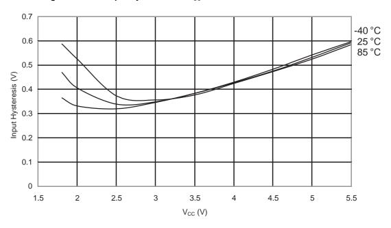
Figure 31-312. ATmega328: Reset Input Threshold Voltage vs.  $V_{CC}(V_{\mathit{HP}}\ I/O\ Pin\ read\ as\ '1')$
