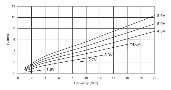
Figure 33-3. ATmega88PA: Active Supply Current vs.  $V_{CC}$  (Internal RC Oscillator, 128kHz)
