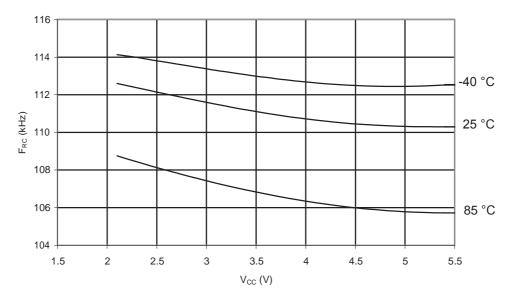
Figure 31-131. ATmega88A: Calibrated 8MHz RC Oscillator Frequency vs. V<sub>CC</sub>
