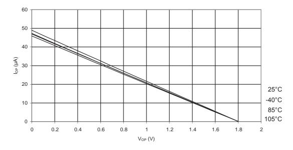
Figure 33-15.ATmega88PA: I/O Pin Pull-up Resistor Current vs. Input Voltage ( $V_{CC} = 2.7V$ )
