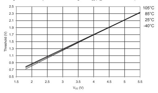
Figure 31-361. ATmega328P: Reset Pin Input Hysteresis vs. V<sub>CC</sub>
