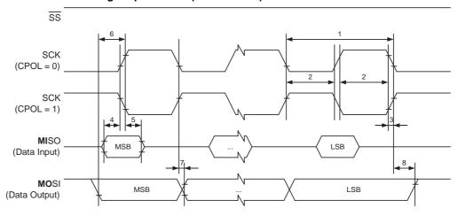
Figure 29-4. SPI Interface Timing Requirements (Slave Mode)
