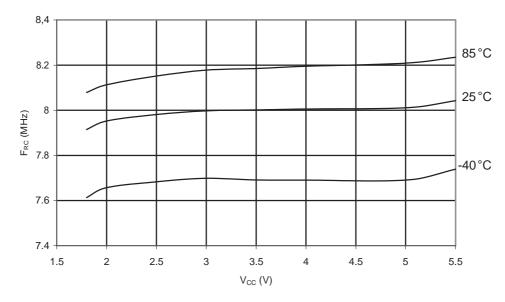
Figure 31-227. ATmega168A: Calibrated 8MHz RC Oscillator Frequency vs. Temperature
