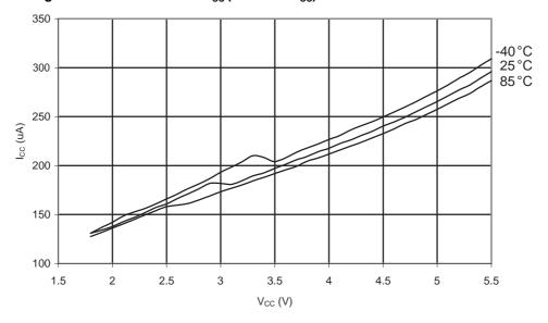
Figure 31-230. ATmega168A: Analog Comparator Current vs.  $V_{\text{CC}}$
