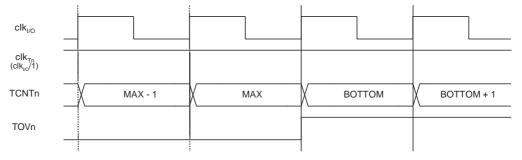
Figure 15-9 shows the same timing data, but with the prescaler enabled.
