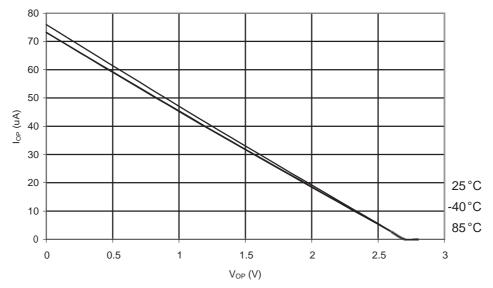
Figure 31-206. ATmega168A: I/O Pin Pull-up Resistor Current vs. Input Voltage (V<sub>CC</sub> = 5 V)
