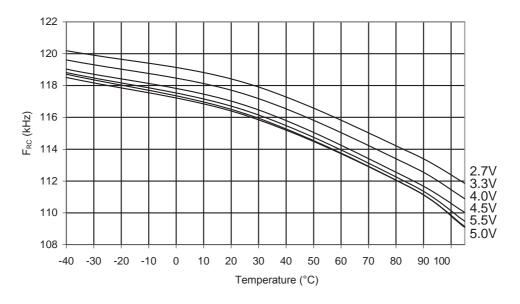
Figure 34-37.ATmega168PA: Watchdog Oscillator Frequency vs. V<sub>CC</sub>
