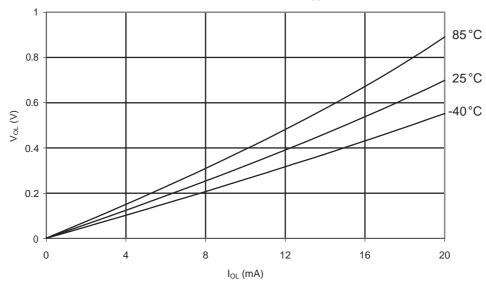
Figure 31-22. ATmega48A: I/O Pin Output Voltage vs. Sink Current (V<sub>CC</sub> = 5 V)
