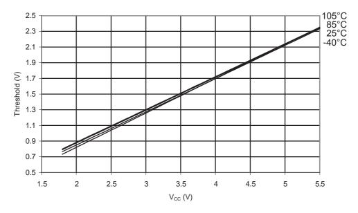
Figure 34-30.ATmega168PA: Reset Pin Input Hysteresis vs. V<sub>CC</sub>
