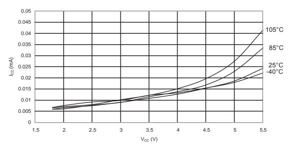
Figure 33-9. ATmega88PA: Idle Supply Current vs. V<sub>CC</sub> (Internal RC Oscillator, 1MHz)
