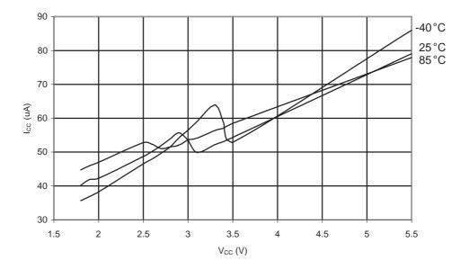
Figure 31-231. ATmega168A: AREF External Reference Current vs. V<sub>CC</sub>
