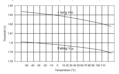
Figure 31-363. ATmega328P: BOD Thresholds vs. Temperature (BODLEVEL is 2.7V)
