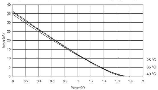
Figure 31-303. ATmega328: Reset Pull-up Resistor Current vs. Reset Pin Voltage (V<sub>CC</sub> = 2.7 V)
