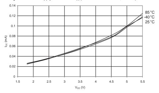
Figure 31-4. ATmega48A: Active Supply Current vs. V<sub>CC</sub> (Internal RC Oscillator, 1MHz)
