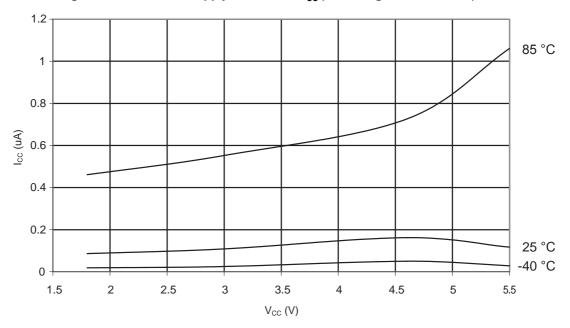
Figure 31-296. ATmega328: Power-Down Supply Current vs. V<sub>CC</sub> (Watchdog Timer Enabled)
