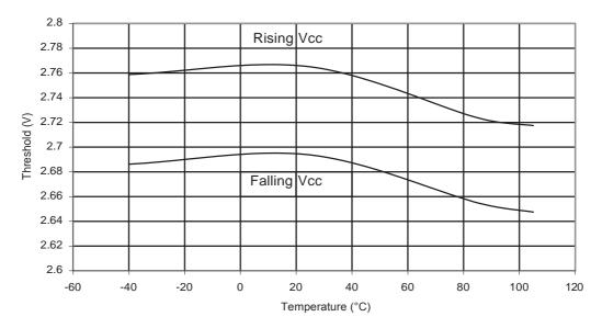
Figure 31-174. ATmega88PA: BOD Thresholds vs. Temperature (BODLEVEL is 4.3V)
