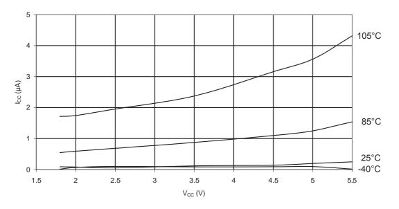
Figure 33-12.ATmega88PA: Power-Down Supply Current vs. V<sub>CC</sub> (Watchdog Timer Enabled)
