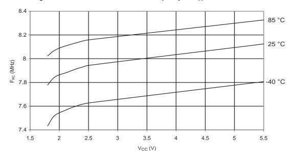
Figure 31-322. ATmega328: Calibrated 8MHz RC Oscillator Frequency vs. Temperature
