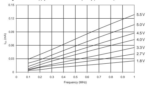
Figure 31-148. ATmega88PA: Idle Supply Current vs. Frequency (1 - 20MHz)
