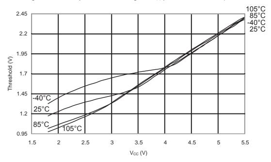
Figure 32-28.ATmega48PA: Reset Input Threshold Voltage vs. V<sub>CC</sub> (V<sub>IL</sub>, I/O Pin read as '0')
