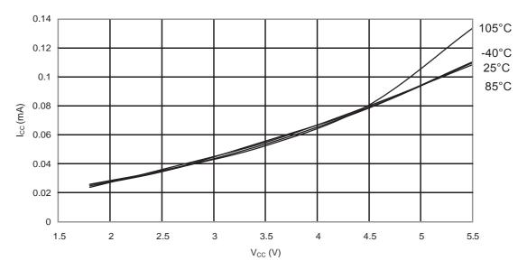
Figure 33-4. ATmega88PA: Active Supply Current vs. V<sub>CC</sub> (Internal RC Oscillator, 1MHz)
