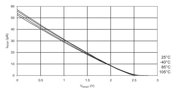
Figure 33-19.ATmega88PA: Reset Pull-up Resistor Current vs. Reset Pin Voltage (V<sub>CC</sub> = 5V)
