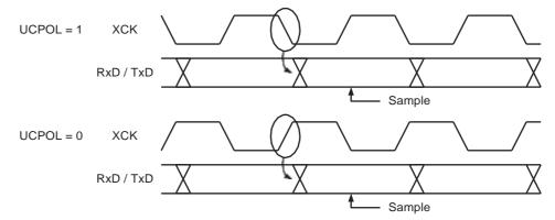
The UCPOLn bit UCRSC selects which XCKn clock edge is used for data sampling and which is used for data change. As Figure 20-3 shows, when UCPOLn is zero the data will be changed at rising XCKn edge and sampled at falling XCKn edge. If UCPOLn is set, the data will be changed at falling XCKn edge and sampled at rising XCKn edge.
