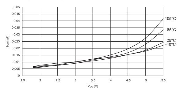
Figure 31-150. ATmega88PA: Idle Supply Current vs. V<sub>CC</sub> (Internal RC Oscillator, 1MHz)
