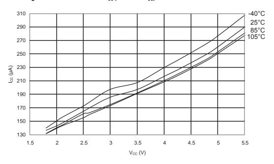
Figure 31-88. ATmega48PA: Analog Comparator Current vs. V<sub>CC</sub>
