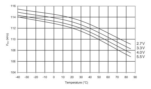
Figure 31-36. ATmega48A: Watchdog Oscillator Frequency vs. V<sub>CC</sub>
