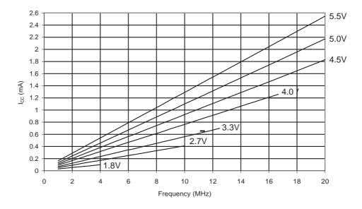
Figure 31-55. ATmega48PA: Idle Supply Current vs. V<sub>CC</sub> (Internal RC Oscillator, 128kHz)
