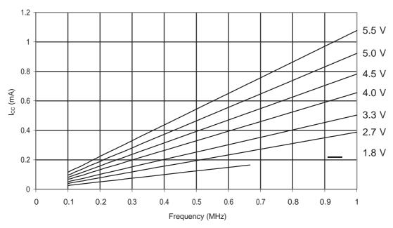
Figure 31-286. ATmega328: Active Supply Current vs. Frequency (1-20MHz)
