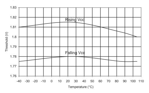
Figure 34-32.ATmega168PA: BOD Thresholds vs. Temperature (BODLEVEL is 2.7V)
