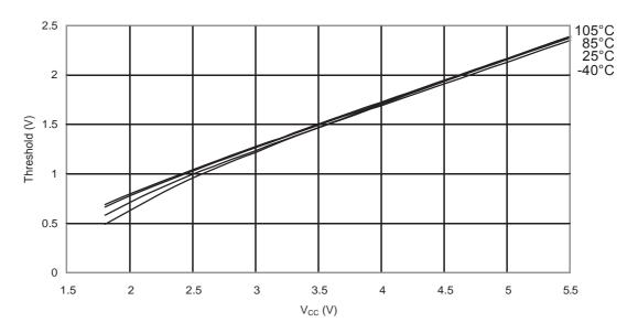
Figure 33-26.ATmega88PA: I/O Pin Input Hysteresis vs. V<sub>CC</sub>
