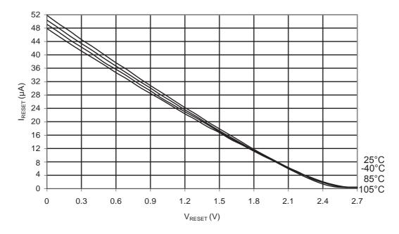
Figure 31-67. ATmega48PA: Reset Pull-up Resistor Current vs. Reset Pin Voltage (V<sub>CC</sub> = 5V)
