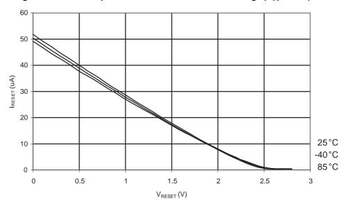
Figure 31-20. ATmega48A: Reset Pull-up Resistor Current vs. Reset Pin Voltage (V<sub>CC</sub> = 5V)
