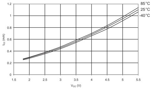
Figure 31-99. ATmega88A: Active Supply Current vs. V<sub>CC</sub> (Internal RC Oscillator, 8MHz)
