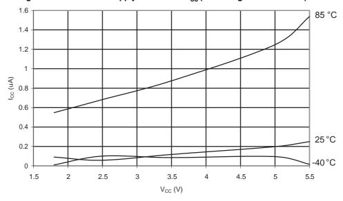
Figure 31-106. ATmega88A: Power-Down Supply Current vs. V<sub>CC</sub> (Watchdog Timer Enabled)
