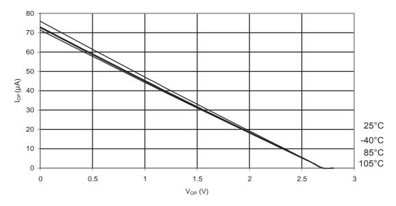
Figure 33-16.ATmega88PA: I/O Pin Pull-up Resistor Current vs. Input Voltage (V<sub>CC</sub> = 5V)
