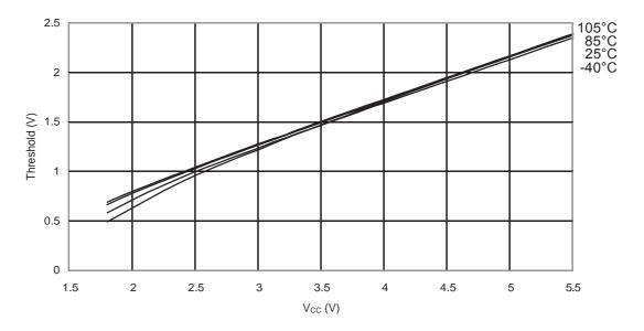
Figure 31-168. ATmega88PA: I/O Pin Input Hysteresis vs. V<sub>CC</sub>
