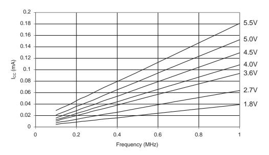
Figure 31-338. ATmega328P: Idle Supply Current vs. Frequency (1-20MHz)
