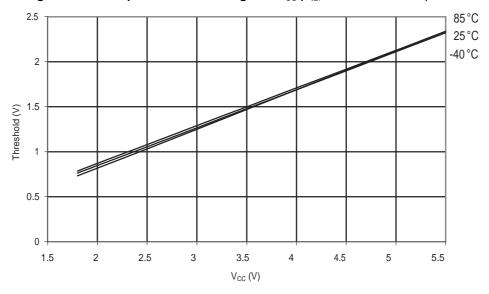
Figure 31-124. ATmega88A: Reset Pin Input Hysteresis vs.  $V_{\text{CC}}$
