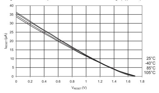
Figure 35-19.ATmega328P: Reset Pull-up Resistor Current vs. Reset Pin Voltage (V<sub>CC</sub> = 2.7V)
