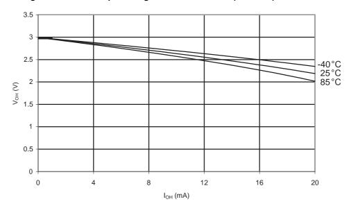
Figure 31-213. ATmega168A: I/O Pin Output Voltage vs. Source Current (V<sub>CC</sub> = 5 V)
