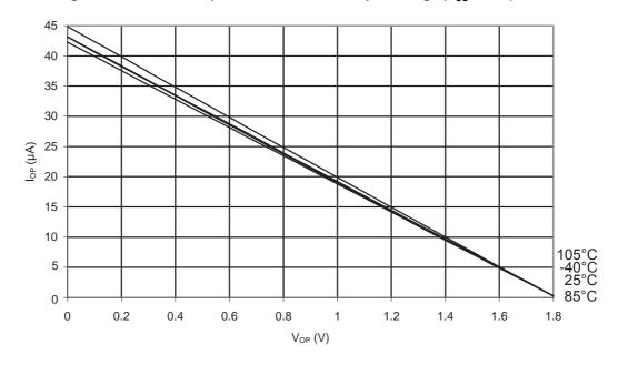
Figure 31-63. ATmega48PA: I/O Pin Pull-up Resistor Current vs. Input Voltage (V<sub>CC</sub> = 2.7V)
