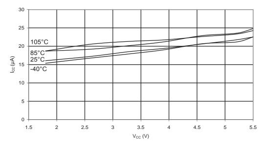
Figure 33-42.ATmega88PA: Programming Current vs. V<sub>CC</sub>
