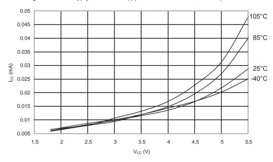
Figure 32-9. ATmega48PA: Idle Supply Current vs. V<sub>CC</sub> (Internal RC Oscillator, 1MHz)
