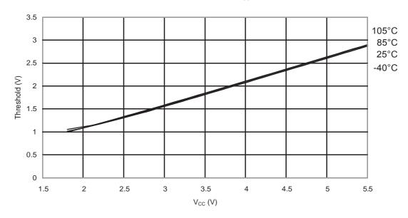
Figure 31-167. ATmega88PA: I/O Pin Input Threshold Voltage vs. V<sub>CC</sub> (V<sub>IL</sub>, I/O Pin read as '0')
