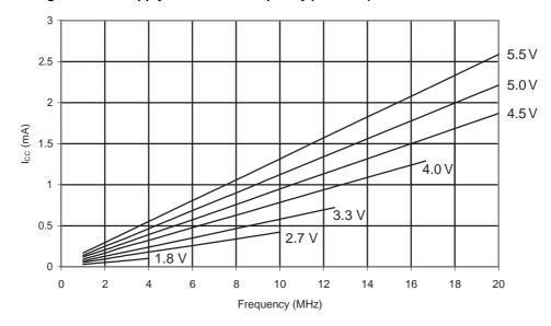
Figure 31-8. ATmega48A: Idle Supply Current vs. V<sub>CC</sub> (Internal RC Oscillator, 128kHz)
