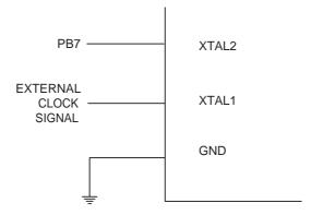
When this clock source is selected, start-up times are determined by the SUT Fuses as shown in Table 9-16.
