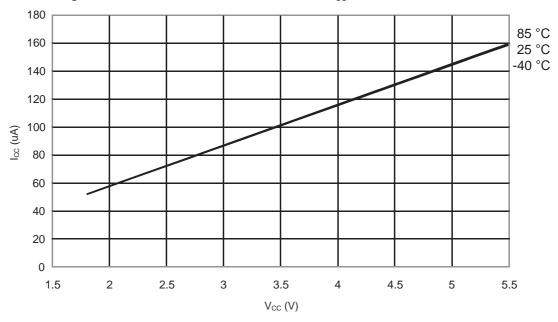
Figure 31-327. ATmega328: Brownout Detector Current vs. V<sub>CC</sub>
