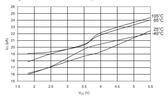
Figure 31-91. ATmega48PA: Programming Current vs. V<sub>CC</sub>
