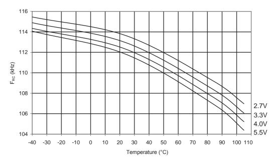
Figure 32-34.ATmega48PA: Watchdog Oscillator Frequency vs. V<sub>CC</sub>
