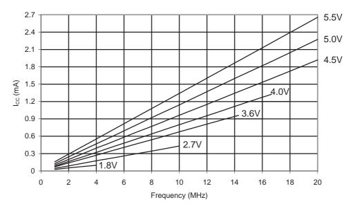
Figure 34-8. ATmega168PA: Idle Supply Current vs. V<sub>CC</sub> (Internal RC Oscillator, 128kHz)
