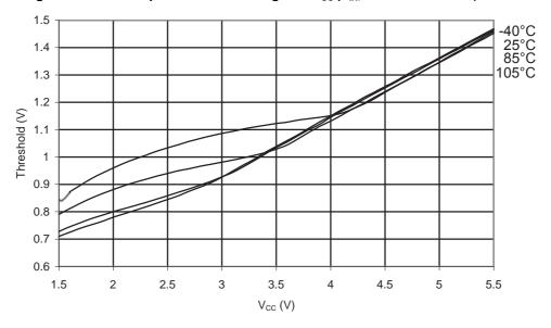
Figure 34-29.ATmega168PA: Reset Input Threshold Voltage vs.  $V_{CC}$  ( $V_{IL}$ , I/O Pin read as '0')
