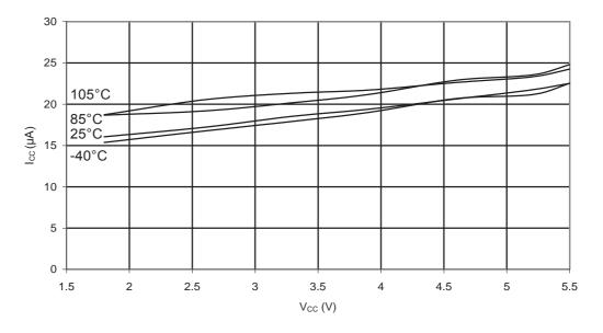
Figure 31-186. ATmega88PA: Programming Current vs. V<sub>CC</sub>
