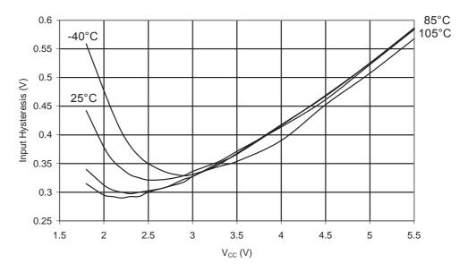
Figure 31-264. ATmega168PA: Reset Input Threshold Voltage vs. V<sub>CC</sub> (V<sub>IH</sub>, I/O Pin read as '1')
