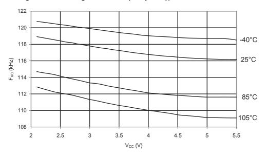
Figure 31-274. ATmega168PA: Calibrated 8MHz RC Oscillator Frequency vs.  $V_{\text{CC}}$
