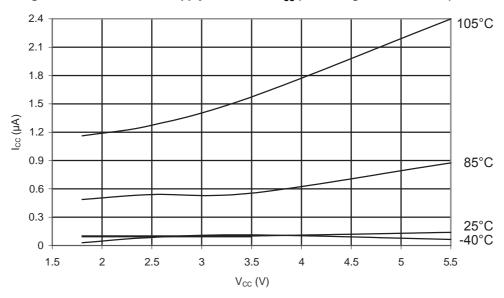
Figure 34-12.ATmega168PA: Power-Down Supply Current vs. V<sub>CC</sub> (Watchdog Timer Enabled)
