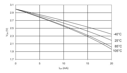
Figure 31-260. ATmega168PA: I/O Pin Output Voltage vs. Source Current (V<sub>CC</sub> = 5V)
