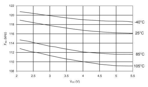
Figure 34-38.ATmega168PA: Calibrated 8MHz RC Oscillator Frequency vs. V<sub>CC</sub>
