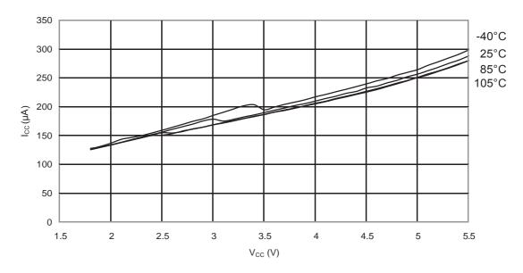
Figure 33-39.ATmega88PA: Analog Comparator Current vs. V<sub>CC</sub>
