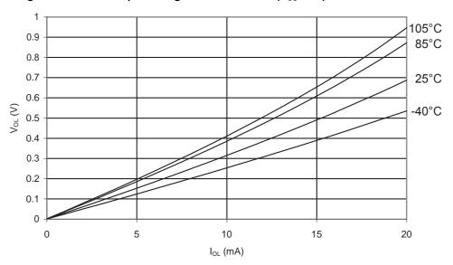
Figure 35-22.ATmega328P: I/O Pin Output Voltage vs. Sink Current (V<sub>CC</sub> = 5V)
