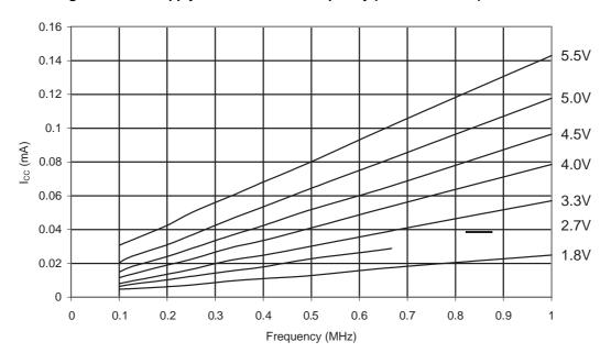
Figure 32-7. ATmega48PA: Idle Supply Current vs. Frequency (1MHz - 20MHz)
