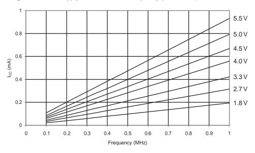
Figure 31-96. ATmega88A: Active Supply Current vs. Frequency (1 - 20MHz)
