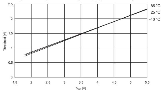
Figure 31-314. ATmega328: Reset Pin Input Hysteresis vs. V<sub>CC</sub>
