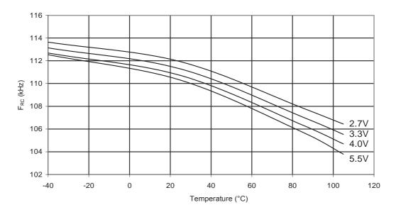
Figure 31-178. ATmega88PA: Watchdog Oscillator Frequency vs. V<sub>CC</sub>
