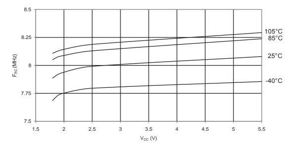
Figure 31-180. ATmega88PA: Calibrated 8MHz RC Oscillator Frequency vs. Temperature
