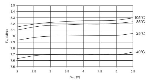
Figure 31-275. ATmega168PA: Calibrated 8MHz RC Oscillator Frequency vs. Temperature
