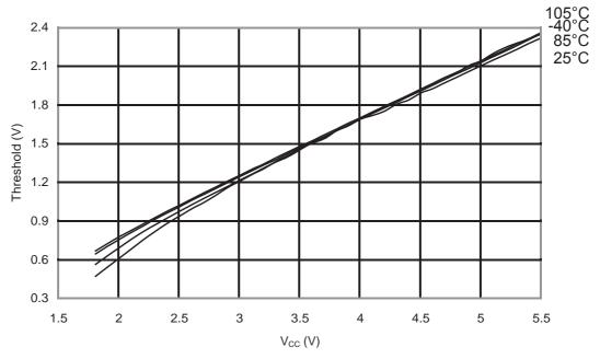
Figure 31-74. ATmega48PA: I/O Pin Input Hysteresis vs. V<sub>CC</sub>
