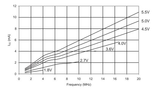
Figure 31-239. ATmega168PA: Active Supply Current vs. V<sub>CC</sub> (Internal RC Oscillator, 128kHz)
