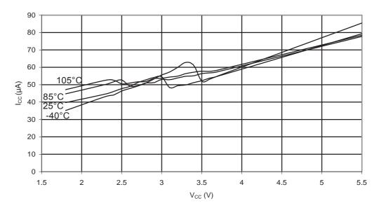
Figure 31-184. ATmega88PA: AREF External Reference Current vs. V<sub>CC</sub>
