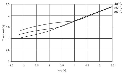
Figure 31-29. )ATmega48A: Reset Input Threshold Voltage vs. V<sub>CC</sub> (V<sub>IL</sub>, I/O Pin read as '0')
