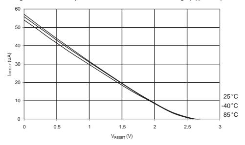
Figure 31-114. ATmega88A: Reset Pull-up Resistor Current vs. Reset Pin Voltage (V<sub>CC</sub> = 5 V)
