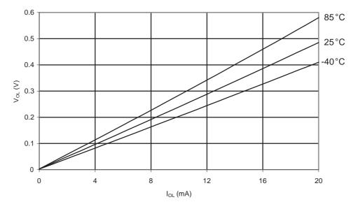
Figure 31-23. ATmega48A: I/O Pin Output Voltage vs. Source Current (Vcc = 3 V)
