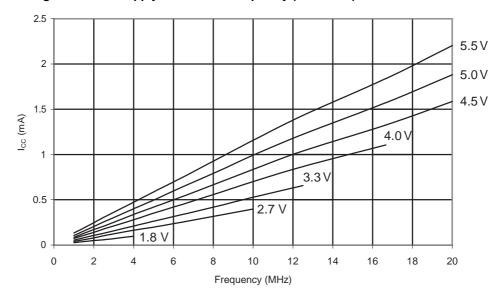
Figure 31-149. ATmega88PA: Idle Supply Current vs. V<sub>CC</sub> (Internal RC Oscillator, 128kHz)
