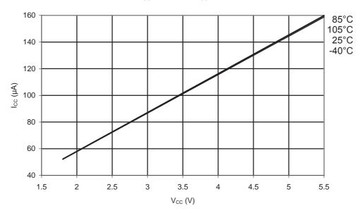
Figure 31-372. ATmega328P: Analog Comparator Current vs. V<sub>CC</sub>
