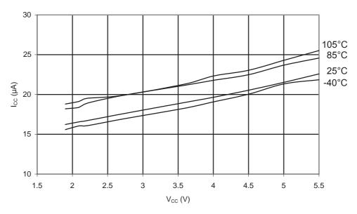
Figure 31-375. ATmega328P: Programming Current vs. V<sub>CC</sub>
