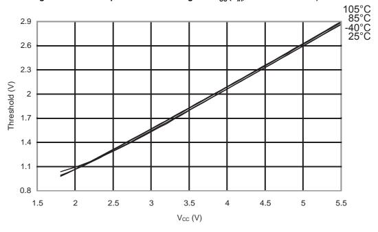
Figure 31-73. ATmega48PA: I/O Pin Input Threshold Voltage vs. V<sub>CC</sub> (V<sub>IL</sub>, I/O Pin read as '0')
