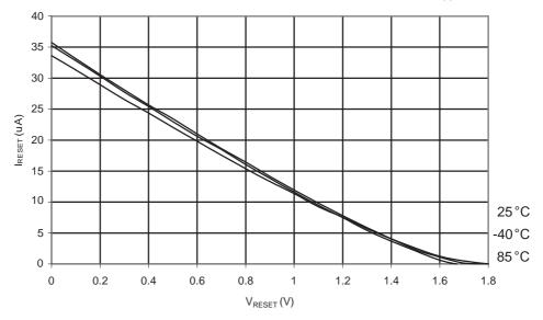
Figure 31-208. ATmega168A: Reset Pull-up Resistor Current vs. Reset Pin Voltage (V<sub>CC</sub> = 2.7 V)
