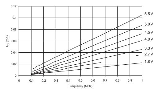
Figure 31-140. ATmega88A: Reset Supply Current vs. Frequency (1 - 20MHz)
