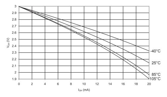
Figure 31-71. ATmega48PA: I/O Pin Output Voltage vs. Source Current (V<sub>CC</sub> = 5V)
