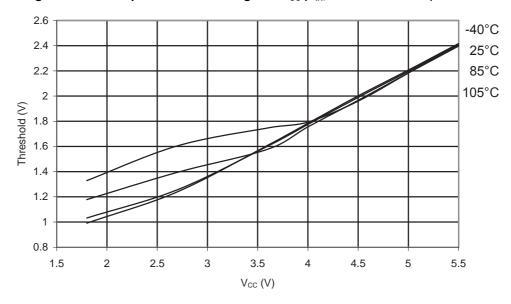
Figure 35-29.ATmega328P: Reset Input Threshold Voltage vs. V<sub>CC</sub> (V<sub>IL</sub>, I/O Pin read as '0')
