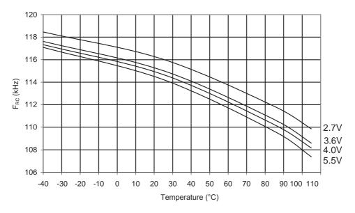
Figure 31-367. ATmega328P: Watchdog Oscillator Frequency vs. V<sub>CC</sub>
