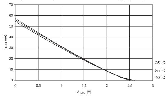
Figure 31-304. ATmega328: Reset Pull-up Resistor Current vs. Reset Pin Voltage (V<sub>CC</sub> = 5 V)
