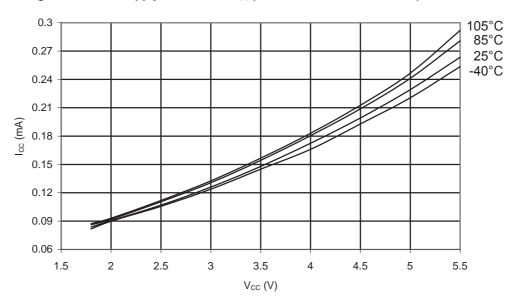
Figure 34-10.ATmega168PA: Idle Supply Current vs. V<sub>CC</sub> (Internal RC Oscillator, 8MHz)
