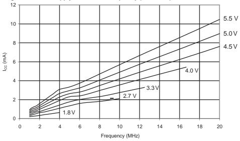
Figure 31-97. ATmega88A: Active Supply Current vs. V<sub>CC</sub> (Internal RC Oscillator, 128kHz)
