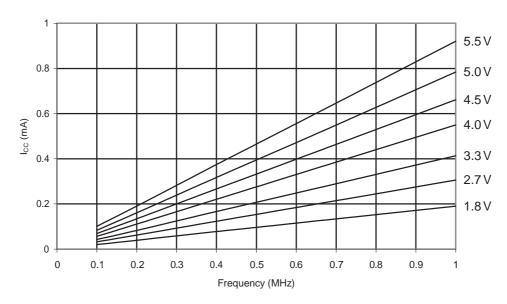
Figure 31-191. ATmega168A: Active Supply Current vs. Frequency (1-20MHz)
