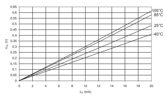
Figure 31-70. ATmega48PA: I/O Pin Output Voltage vs. Source Current (Vcc = 3V)
