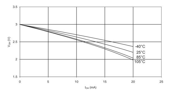
Figure 33-23.ATmega88PA: I/O Pin Output Voltage vs. Source Current (V<sub>CC</sub> = 5V)
