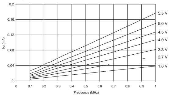
Figure 31-291. ATmega328: Idle Supply Current vs. Frequency (1-20MHz)
