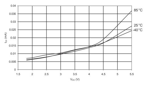
Figure 31-198. ATmega168A: Idle Supply Current vs. V<sub>CC</sub> (Internal RC Oscillator, 1MHz)
