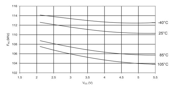
Figure 33-35.ATmega88PA: Calibrated 8MHz RC Oscillator Frequency vs. V<sub>CC</sub>
