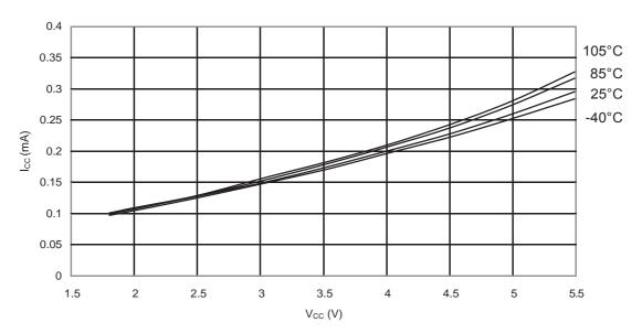
Figure 33-10.ATmega88PA: Idle Supply Current vs. V<sub>CC</sub> (Internal RC Oscillator, 8MHz)
