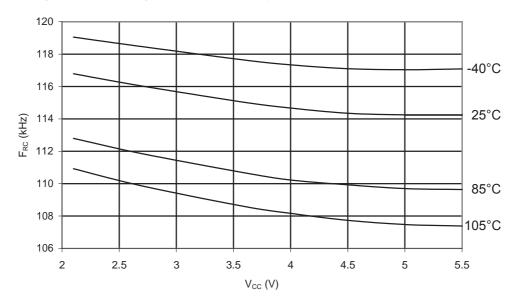
Figure 35-37.ATmega328P: Calibrated 8 MHz RC Oscillator Frequency vs.  $V_{\rm CC}$
