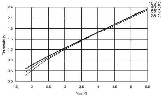
Figure 32-26.ATmega48PA: I/O Pin Input Hysteresis vs. V<sub>CC</sub>
