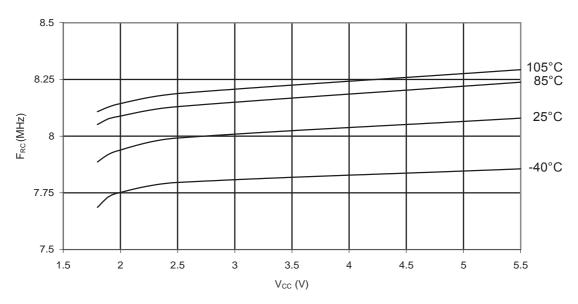
Figure 33-36.ATmega88PA: Calibrated 8MHz RC Oscillator Frequency vs. Temperature
