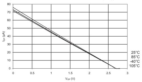
Figure 31-253. ATmega168PA: I/O Pin Pull-up Resistor Current vs. Input Voltage (V<sub>CC</sub> = 5V)
