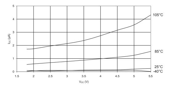
Figure 31-153. ATmega88PA: Power-Down Supply Current vs. V<sub>CC</sub> (Watchdog Timer Enabled)
