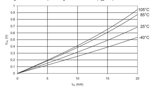
Figure 31-353. ATmega328P: I/O Pin Output Voltage vs. Sink Current (V<sub>CC</sub> = 5V)
