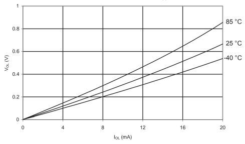
Figure 31-211. ATmega168A: I/O Pin Output Voltage vs. Sink Current (V<sub>CC</sub> = 5 V)
