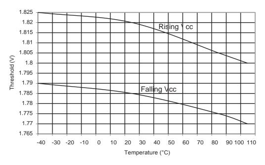
Figure 32-31.ATmega48PA: BOD Thresholds vs. Temperature (BODLEVEL is 2.7V)
