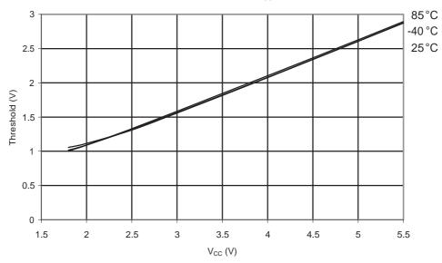
Figure 31-120. ATmega88A: I/O Pin Input Threshold Voltage vs.  $V_{CC}$  ( $V_{IL}$ , I/O Pin read as '0'
