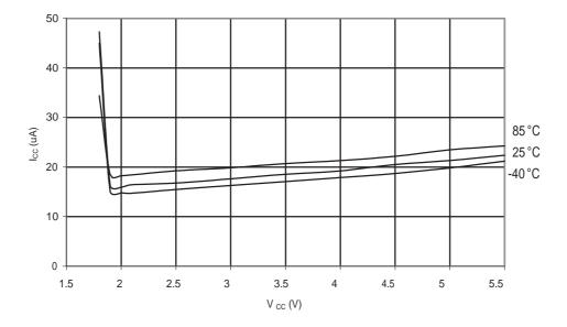
Figure 31-138. ATmega88A: Programming Current vs. V<sub>CC</sub>
