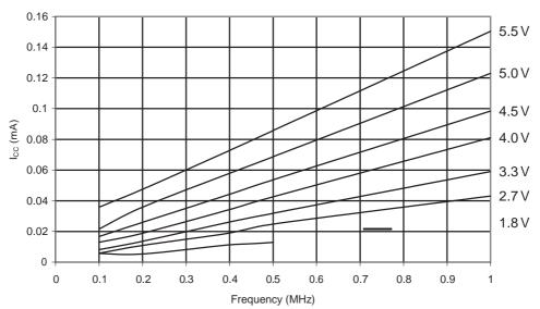
Figure 31-7. ATmega48A: Idle Supply Current vs. Frequency (1-20MHz)
