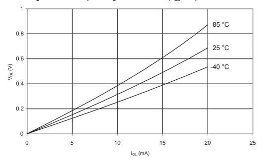
Figure 31-306. ATmega328: I/O Pin Output Voltage vs. Sink Current ( $V_{CC} = 5 \text{ V}$ )
