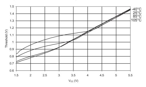
Figure 31-265. ATmega168PA: Reset Input Threshold Voltage vs. V<sub>CC</sub> (V<sub>IL</sub>, I/O Pin read as '0')
