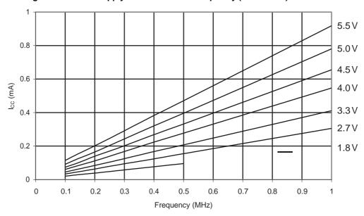
Figure 31-49. ATmega48PA: Active Supply Current vs. Frequency (1-20MHz)
