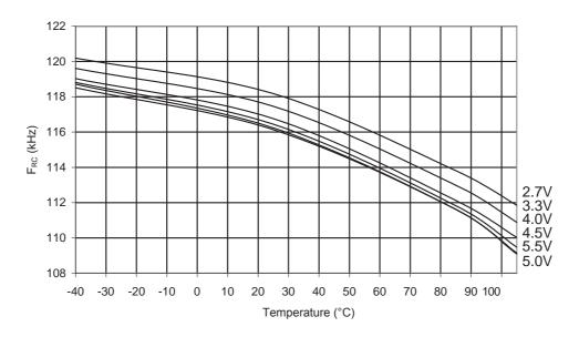
Figure 31-273. ATmega168PA: Watchdog Oscillator Frequency vs. V<sub>CC</sub>
