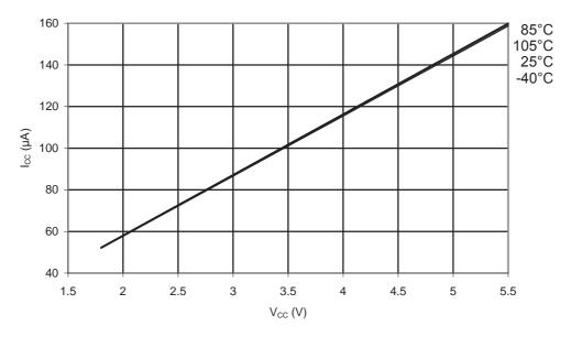
Figure 35-41.ATmega328P: Analog Comparator Current vs. V<sub>CC</sub>
