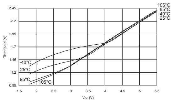
Figure 31-76. ATmega48PA: Reset Input Threshold Voltage vs. V<sub>CC</sub> (V<sub>IL</sub>, I/O Pin read as '0')
