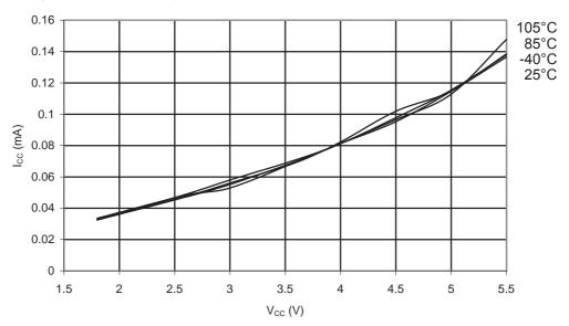
Figure 35-4. ATmega328P: Active Supply Current vs. V<sub>CC</sub> (Internal RC Oscillator, 1MHz)
