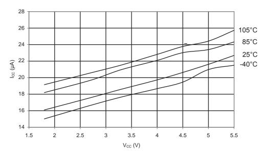
Figure 31-281. ATmega168PA: Programming Current vs. V<sub>CC</sub>
