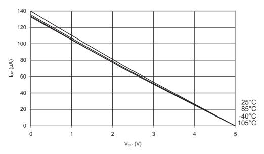
Figure 34-18.ATmega168PA: Reset Pull-up Resistor Current vs. Reset Pin Voltage  $(V_{CC} = 1.8V)$
