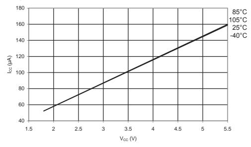
Figure 35-43.ATmega328P: Brownout Detector Current vs. V<sub>CC</sub>
