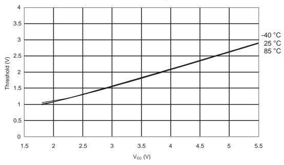
Figure 31-310. ATmega328: I/O Pin Input Threshold Voltage vs. V<sub>CC</sub> (V<sub>IL</sub>, I/O Pin read as '0')
