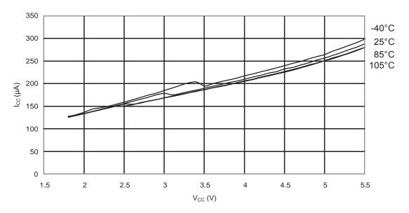
Figure 31-183. ATmega88PA: Analog Comparator Current vs.  $V_{\text{CC}}$
