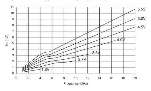
Figure 31-50. ATmega48PA: Active Supply Current vs. V<sub>CC</sub> (Internal RC Oscillator, 128kHz)
