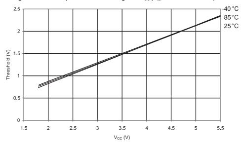
Figure 31-219. ATmega168A: Reset Pin Input Hysteresis vs. V<sub>CC</sub>
