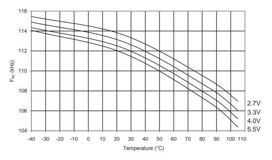
Figure 31-83. ATmega48PA: Watchdog Oscillator Frequency vs.  $V_{\text{CC}}$
