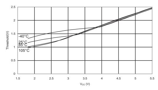
Figure 33-28.ATmega88PA: Reset Input Threshold Voltage vs. V<sub>CC</sub> (V<sub>IL</sub>, I/O Pin read as '0')
