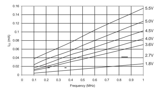
Figure 31-243. ATmega168PA: Idle Supply Current vs. Frequency (1-20MHz)
