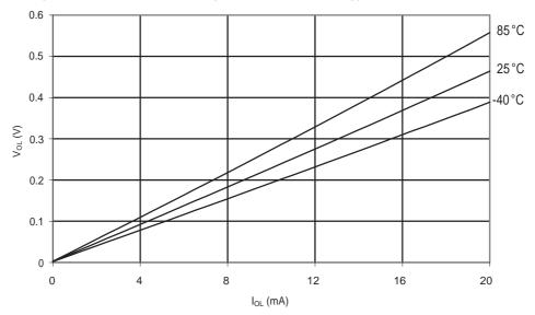
Figure 31-117. ATmega88A: I/O Pin Output Voltage vs. Source Current (Vcc = 3 V)
