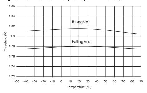
Figure 31-221. ATmega168A: BOD Thresholds vs. Temperature (BODLEVEL is 2.7 V)
