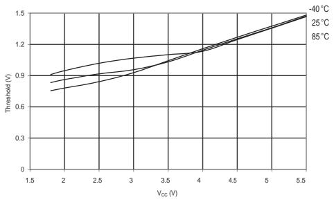
Figure 31-123. ATmega88A: Reset Input Threshold Voltage vs. V<sub>CC</sub> (V<sub>IL</sub>, I/O Pin read as '0')
