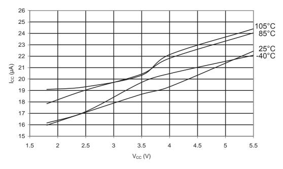
Figure 32-42.ATmega48PA: Programming Current vs. V<sub>CC</sub>
