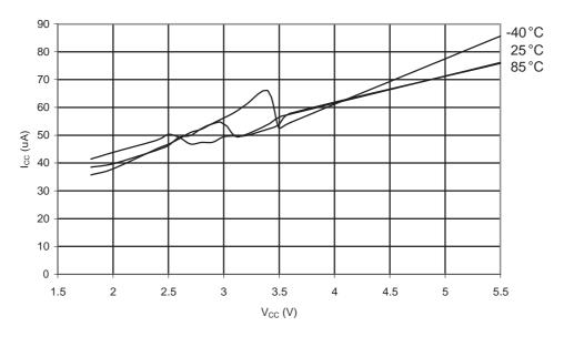
Figure 31-42. ATmega48A: AREF External Reference Current vs. V<sub>CC</sub>
