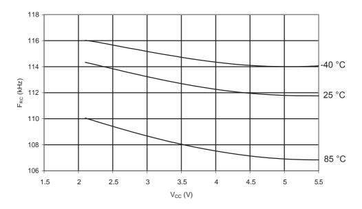
Figure 31-37. ATmega48A: Calibrated 8MHz RC Oscillator Frequency vs. V<sub>CC</sub>
