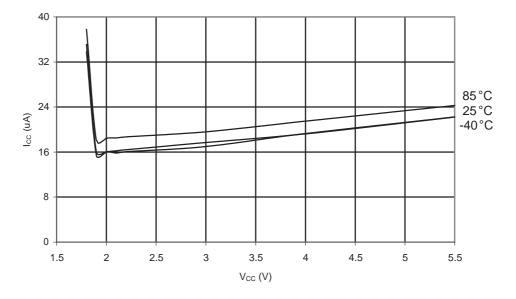
Figure 31-44. ATmega48A: Programming Current vs. V<sub>CC</sub>
