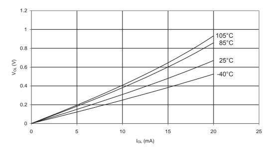
Figure 33-21.ATmega88PA: I/O Pin Output Voltage vs. Sink Current (V<sub>CC</sub> = 5V)
