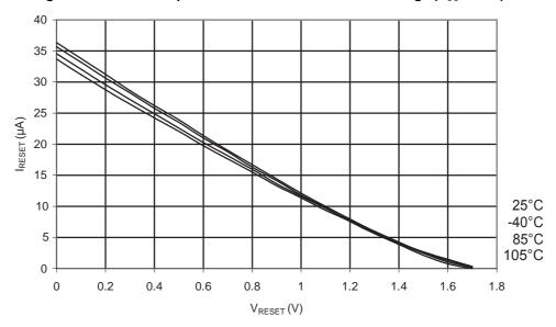
Figure 31-350. ATmega328P: Reset Pull-up Resistor Current vs. Reset Pin Voltage (V<sub>CC</sub> = 2.7V)
