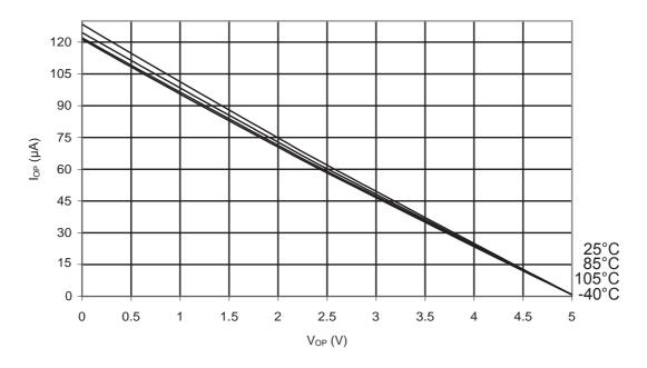
Figure 32-17.ATmega48PA: Reset Pull-up Resistor Current vs. Reset Pin Voltage (V<sub>CC</sub> = 1.8V)
