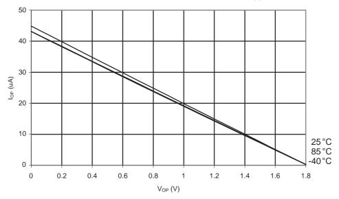
Figure 31-16. ATmega48A: I/O Pin Pull-up Resistor Current vs. Input Voltage (V<sub>CC</sub> = 2.7 V)
