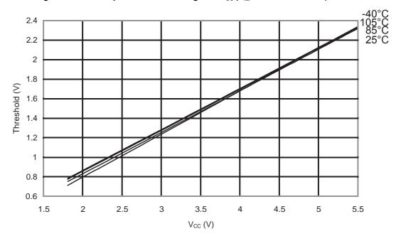
Figure 32-29.ATmega48PA: Reset Pin Input Hysteresis vs. V<sub>CC</sub>
