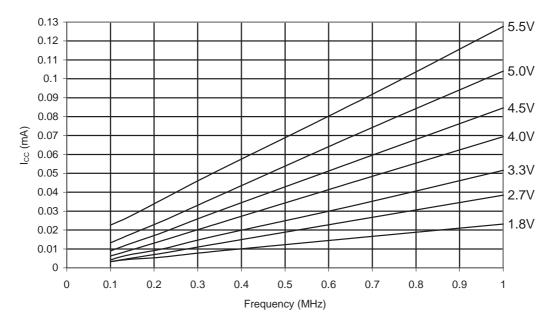
Figure 32-44.ATmega48PA: Reset Supply Current vs. Frequency (1MHz- 20MHz)
