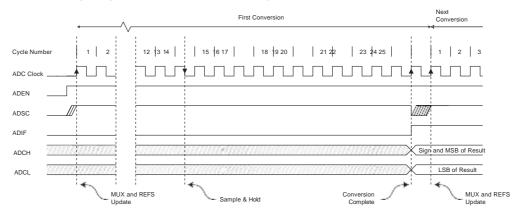
Figure 24-5. ADC Timing Diagram, Single Conversion
