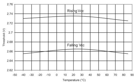
Figure 31-222. ATmega168A: BOD Thresholds vs. Temperature (BODLEVEL is 4.3 V)
