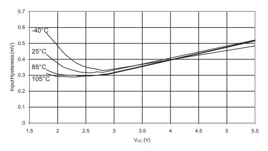
Figure 31-169. ATmega88PA: Reset Input Threshold Voltage vs. V<sub>CC</sub> (V<sub>III</sub>, I/O Pin read as '1')
