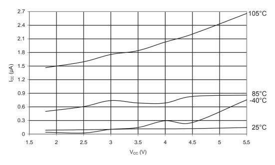
Figure 31-59. ATmega48PA: Power-Down Supply Current vs. V<sub>CC</sub> (Watchdog Timer Enabled)
