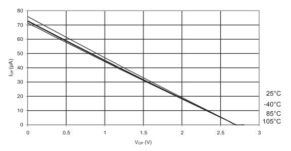
Figure 31-158. ATmega88PA: I/O Pin Pull-up Resistor Current vs. Input Voltage (V<sub>CC</sub> = 5V)
