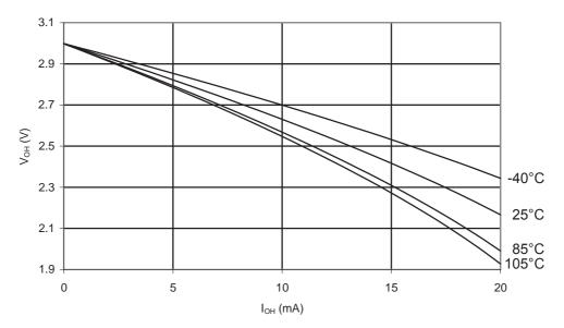
Figure 35-24.ATmega328P: I/O Pin Output Voltage vs. Source Current (V<sub>CC</sub> = 5V)
