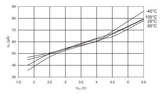
Figure 34-43.ATmega168PA: AREF External Reference Current vs. V<sub>CC</sub>
