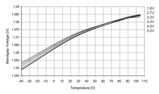
Figure 31-176. ATmega88PA: Bandgap Voltage vs. V<sub>CC</sub>
