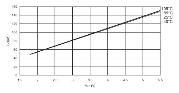
Figure 33-41.ATmega88PA: Brownout Detector Current vs. V<sub>CC</sub>
