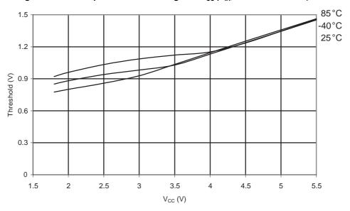
Figure 31-218. ATmega168A: Reset Input Threshold Voltage vs. V<sub>CC</sub> (V<sub>IL</sub>, I/O Pin read as '0')
