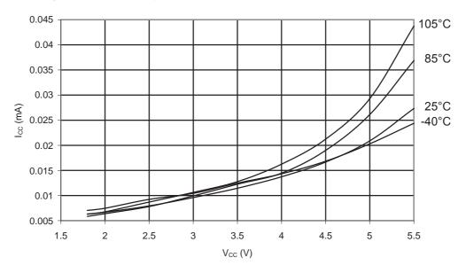
Figure 31-245. ATmega168PA: Idle Supply Current vs. V<sub>CC</sub> (Internal RC Oscillator, 1MHz)
