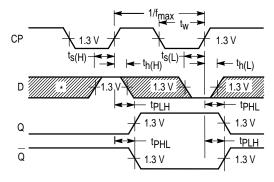
\*The shaded areas indicate when the input is permitted to change for predictable output performance.
