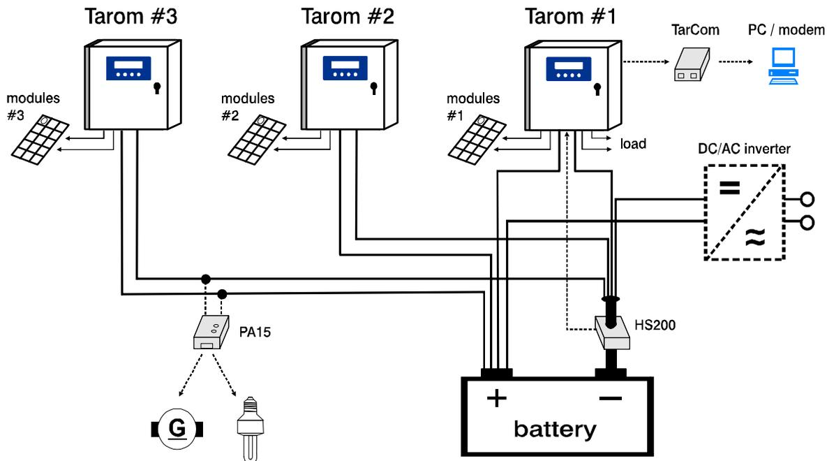
In a photovoltaic system several PowerTarom regulators can charge a battery simultaneously. Please note the following notes for an optimal installation:
