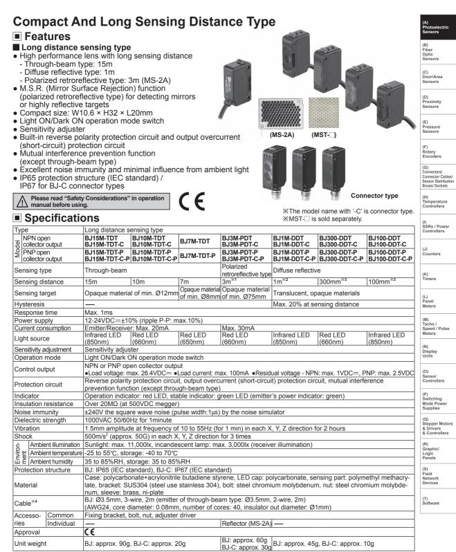
\*1: The sensing distance is specified with using the MS-2A reflector. The distance between the sensor and the reflector should be set over 0.1m. The sensing distance is extended from 0.1 to 4m or 0.1 to 5m when using optional reflector MS-2S or MS-3S. When using reflective tapes, the reflectivity will vary by the size of the tape. Please refer to the "I Reflectivity By Reflective Tape Model" table before using the tapes. \*22: Non-glossy white paper 300×300mm.
