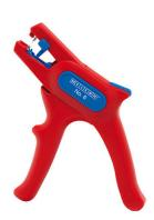
The WEICON Wire Stripper No. 6 has an adjustable length stop from 5-12 mm. This allows all flexible and solid conductors of 0.2-6.0 mm² (24 -10 AWG) to be stripped. The length stop can be removed if required. This fully-insulated tool is subject to routine testing in accordance with the VDE regulation as per IEC 60900:2004 and can withstand a voltage of 1000 volts.
