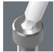
The spherical drive profile means that it is possible to swivel the axis of the tool to that of the screw, and therefore enable angled, "around-the-corner" screwdriving iobs.
