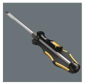
A hexagon blade made out of highquality bit material extends right through the handle – thereby ensuring full transfer of force, even when struck with a hammer. The ductile tempered material prevents the blade from splintering or breaking. A line of the second se
