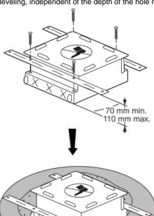
After having broken the concrete in the desired area, the back box can be installed from above (resting on the existing screed by means of 2 sleepers, not provided).
