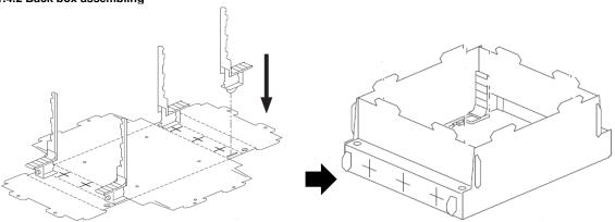
Clips the 4 rigid plastic parts into the dedicated locations then fold and assemble the back box
