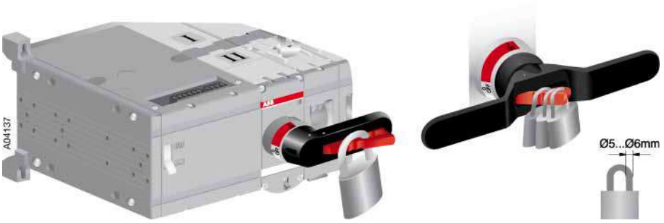
Figure 6.8 Locking the manual operation
