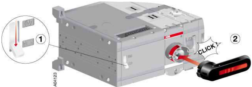
Figure 3.3 Operating the motorized change-over switch manually
