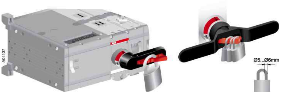
Figure 3.4 Locking the manual operation
