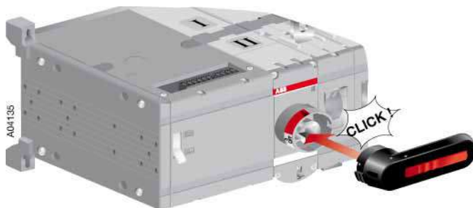
Figure 6.6 Attaching the handle
