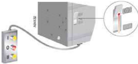
Figure 6.2 Motor/Manual selection switch in the Motor (M) position
