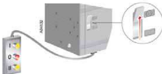
Figure 6.2 Motor/Manual selection switch in the Motor (M) position
