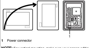
When installing this product in a slanted position, the product face should not incline more than 30°.
