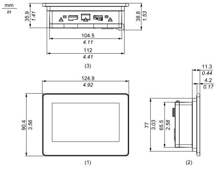
**NOTE:** External view is shown using first angle projection method.
