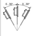
When installing this product in a slanted position with an incline more than  $30^\circ$ , the ambient temperature must not exceed  $40^\circ$ C ( $104^\circ$ F). You may need to use forced air cooling (fan, A/C) to ensure the ambient operating temperature is  $40^\circ$ C or less ( $104^\circ$ F or less).
