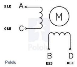
Bipolar stepper motor wiring diagram.
