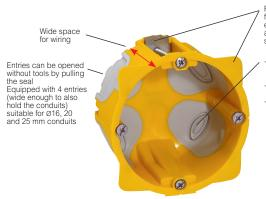
Reinforced wide flange and clamps ensure boxes are held in place securely
