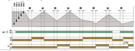
Filling tank and draining well function + alarm
