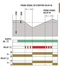
Delay for LVM30 only.Changeover contact (SPDT) for LVM30 only.
