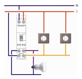
. 4 "NO" pulse operated latching relay
