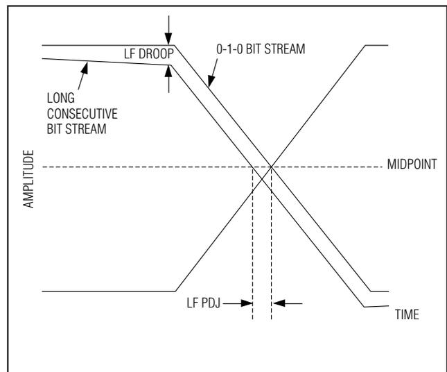
Figure 9. Pattern-Dependent Jitter Due to Low-Frequency Cutoff
