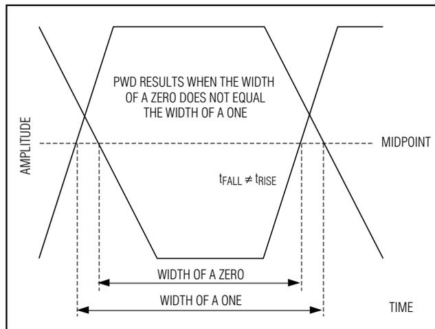
Figure 11. Pulse-Width Distortion
