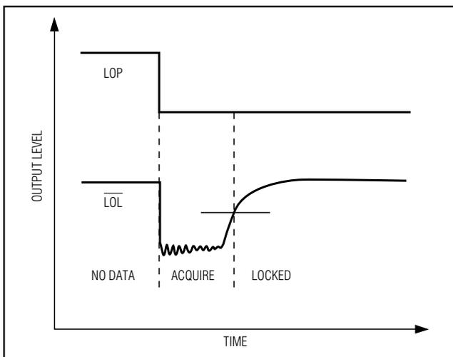
Figure 4. Loss-of-Lock Output
