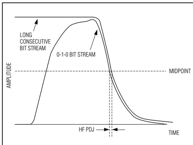
Figure 10. Pattern-Dependent Jitter Due to High-Frequency Roll-off
