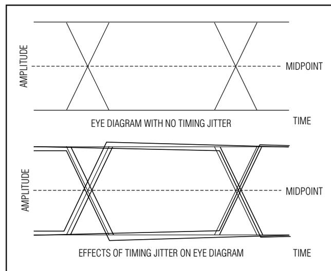
Figure 7. Eye Diagram With and Without Timing Jitter
