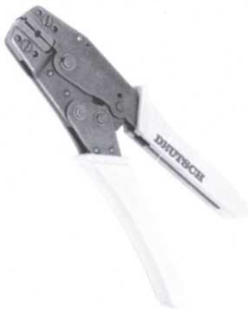
DTT-20-0* Hand Crimp Tool Stamped & Formed Contacts
