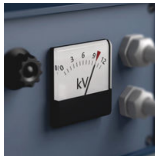
The individual testing of the Zyklop tools for electricians at 10,000 volts, in accordance with IEC 60900, guarantees safe working under voltages up to 1,000 volts.
