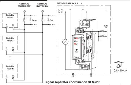
In the bistable control systems signal separators can be used to divide control signals into particular relay groups.
