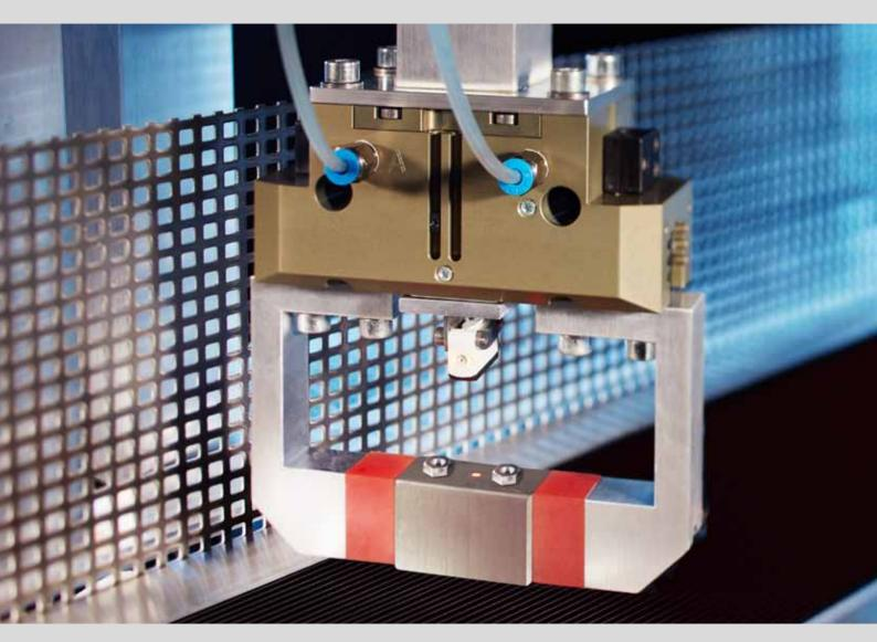
In the robot's arm: Thanks to its miniaturised housing and low weight the sensors of the F 10 series are predestined for use where space is very limited – integrated in a robot arm, for example.
