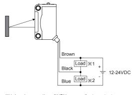
X1: Load connection of NPN open collector output
