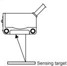
If the sensing target has a glossy surface, mount the sensor at a 5 to 10° angle as shown in the figure. Check to see that there is no influence from background objects.
