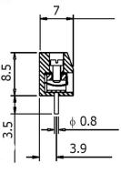
Recommended PCB holes diameter: f 1.2 mm to f 1.4 mm
