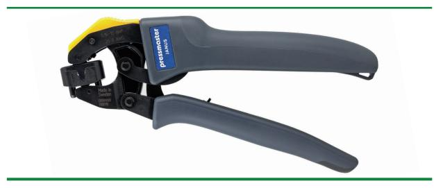
Janus, the lightest and most compact crimp tool of its type, has a rotatable die set so that the ferrule can be inserted into the front or side of the tool to suit cabinet and bench working respectively. The tool is self-adjusting to produce a trapezoid shaped crimp profile on wire ferrules 0.14–10.0 mm<sup>2</sup>/AWG 26–8 (produced to DIN 46228-parts 1 and 4 or UL 486F).
