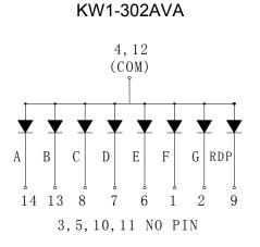
Internal Circuit Diagram (Common Cathode)
