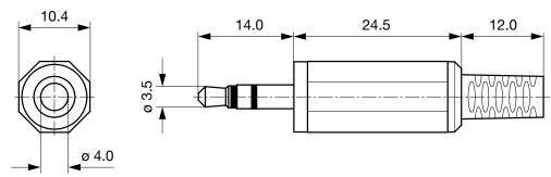
Cable diameter max. 4.0 mm
