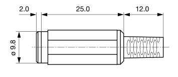
Cable diameter max. 4.0 mm
