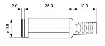
Cable diameter max. 4.0 mm
