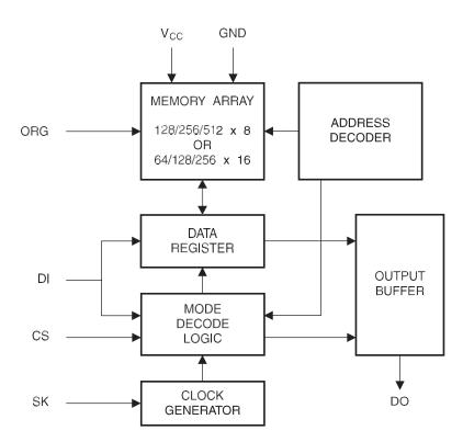
Note: 1. When the ORG pin is connected to V<sub>CC</sub>, the x 16 organization is selected. When it is connected to ground, the x 8 organization is selected. If the ORG pin is left unconnected, then an internal pullup device (of approximately 1 MΩ) will select the x 16 organization. This feature is not available on 1.8V devices.
