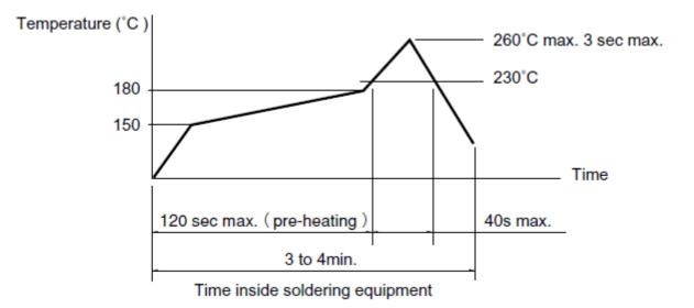
(1) The above temperature shall be measured of the top of switch. There are cases where PC board's temperature greatly differs from that of the switch, depending on the material, size, thickness of PC board's and others. Care, should be taken to prevent the switch's surface temperature from exceeding 260°C.
