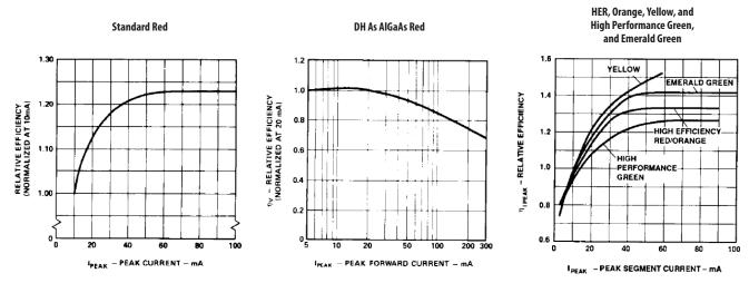
Figure 4. Relative efficiency (luminous intensity per unit current) vs. peak current (non-resistor lamps).
