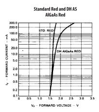
Figure 2. Forward current vs. forward voltage (non-resistor lamp).
