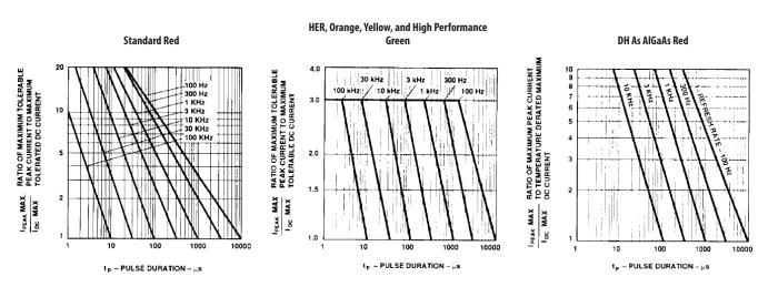
Figure 6. Maximum tolerable peak current vs. pulse duration (I<sub>DC</sub> MAX as per MAX ratings) (non-resistor lamps).
