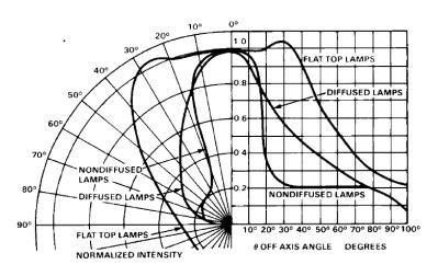
Figure 9. Relative intensity vs. angular displacement.
