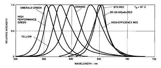
Figure 1. Relative intensity vs. wavelength.
