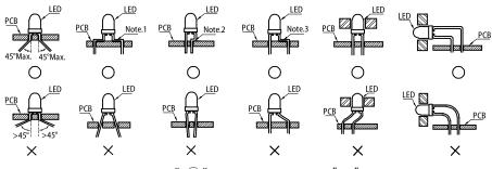
" Correct mounting method " x " Incorrect mounting method
