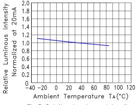
Fig.5 Relative Luminous Intensity VS. Ambient Temperature
