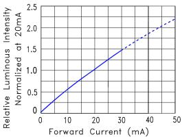
Fig.4 Relative Luminous Intensity vs. Forward Current
