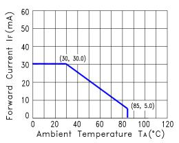
Fig.2 Forward Current Derating Curve
