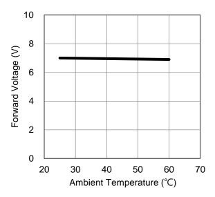
Fig 6. Ambient Temperature vs. Forward Voltage
