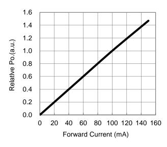
Fig 2. Forward Current vs. Relative Radiant Flux
