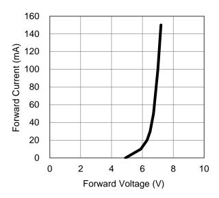
Fig 3. Forward Voltage vs Forward Current
