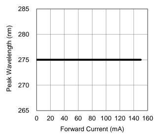
Fig 1. Forward Current vs. Peak Wavelength
