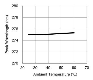
Fig 5. Ambient Temperature vs. Peak Wavelength
