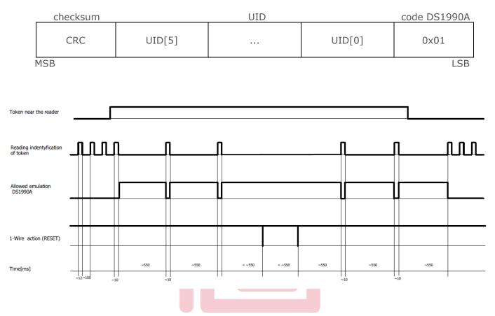
1. The reader is waiting for the proximity of the token (card) trying to read it at a frequency of about 6 times per second. ( $\sim$  12 ms [checking the presence of the card] +  $\sim$  150 ms [gap between successive checks]).
