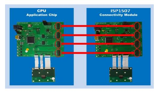
For SPI interface, connect all the following pins on the highlighted connectors:
