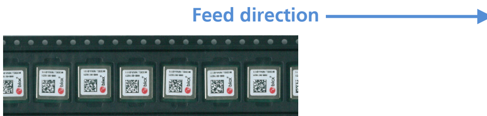
Figure 8: Orientation of NINA-W131 module on tape
