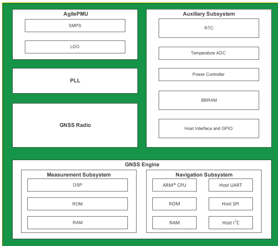
FIGURE 2 – SiRFstarV™ 5e GNSS SoC BLOCK DIAGRAM
