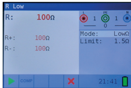
Figure 4 7: Examples of R Low resistance measurement results
