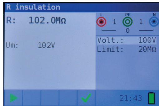
Figure 4 3: Example of insulation resistance measurement results
