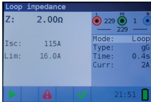
Figure 4 23: Example of loop impedance measurement results
