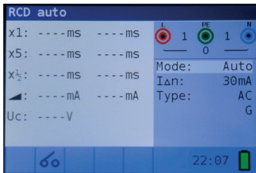
Figure 4 18: RCD autotest menu
