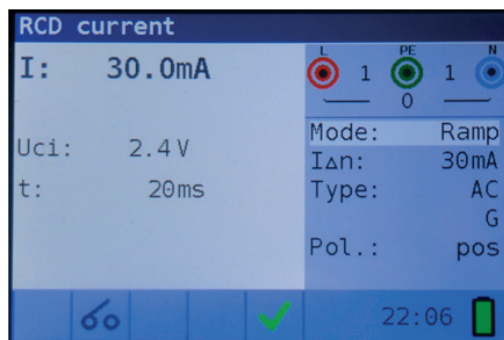
Figure 4 17: Example of trip-out current measurement result
