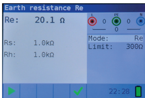
Figure 4 38: Example of resistance to earth measurement results
