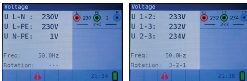
Figure 4.34: Examples of voltage and frequency measurements
