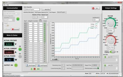
PC software is provided for front panel emulation, generating and executing test sequences or logging measurement data without the need to write source code.
