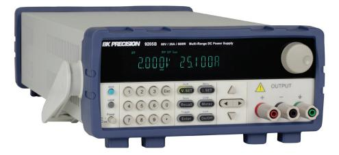
The 9200B Series can replace multiple supplies on your bench or in your rack. Unlike conventional supplies with fixed output ratings, the 9200B Series automatically recalculates voltage and current limits for each setting, providing maximum output power in any Volt/Amp combination within the rated voltage and current limits.
