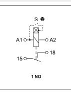
The control terminal S is activated by connection to A1 terminal via the external control contact S.
