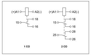
**Note**: the indicated polarity of the supply refers only to the relays RPC-...-UNI.
