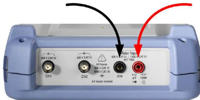
Figure 6-1: Meter inputs to connect test leads
