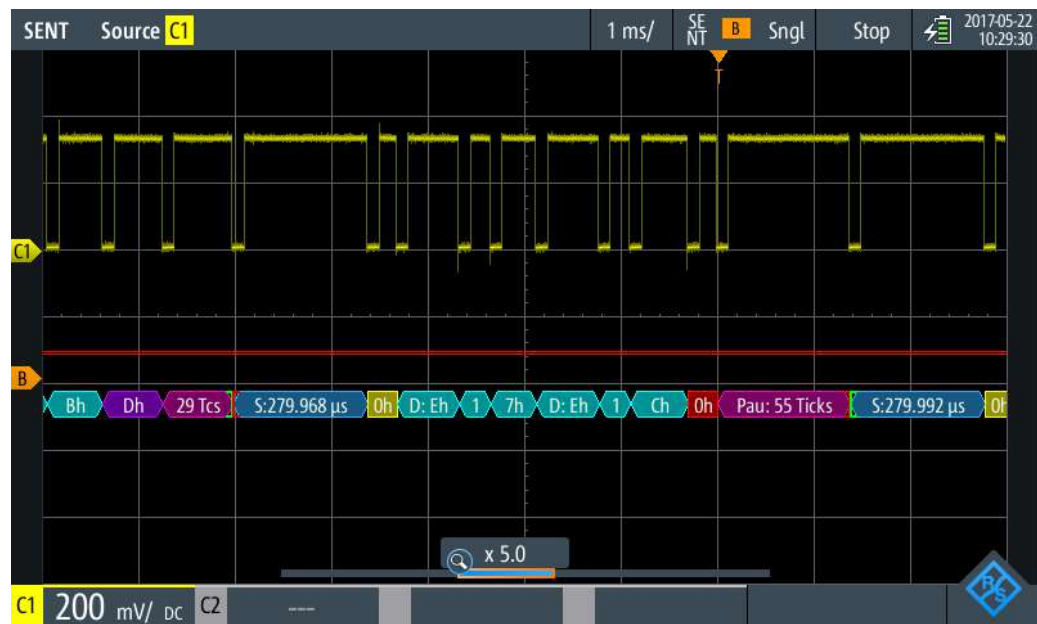
Figure 8-30: Comb display of a decoded SENT signal, triggered on fast CRC
