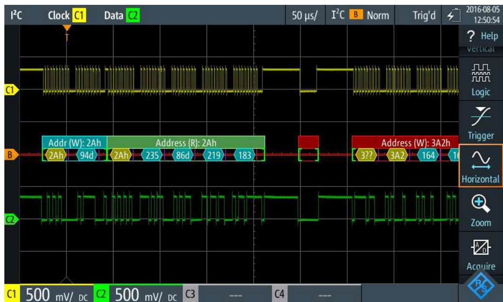
Figure 8-9: Comb display of a decoded I 2 C signal, triggered on address 2A (hex)
