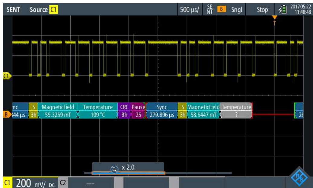
Figure 8-28: SENT decode results with label list translation
