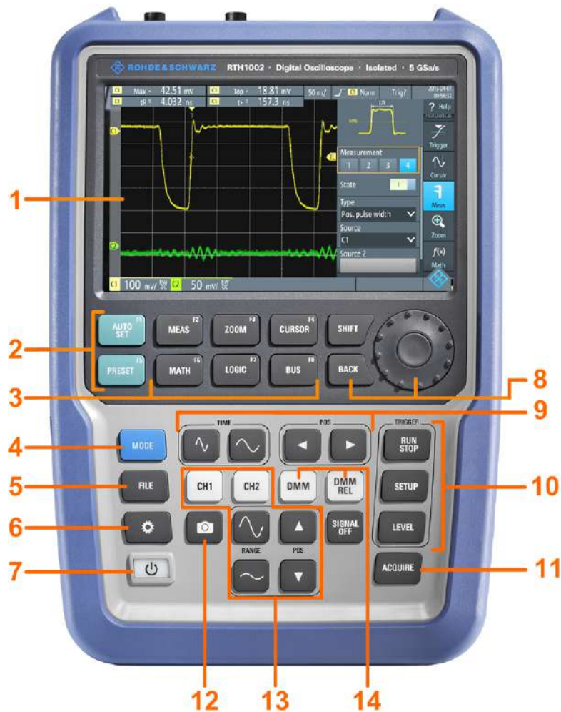
Figure 1-3: Front panel of the R&S RTH1002
