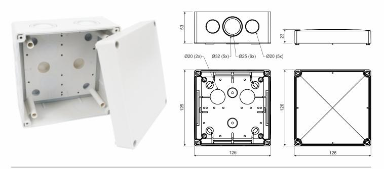
intended for installation in environments that require IP 66 protection description: made from UV-resistant stable integrated knockouts for mounting on base perfect sealing of cables and pipes integrated O-ring to install cable glands intended for direct installation on the surface without having to support with insulating pad stainless steel screws for lid installation the option to install special terminal block 7x inlets with Ø20 mm; 6x Ø25 mm; 5x Ø32 mm
