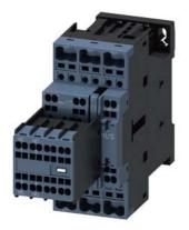
power contactor, AC-3e/AC-3, 25 A, 11 kW / 400 V, 3-pole, 24 V AC, 50/60 Hz, auxiliary contacts: 2 NO + 2 NC, spring-loaded terminal, removable auxiliary switch
