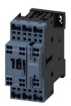
power contactor, AC-3e/AC-3, 25 A, 11 kW / 400 V, 3-pole, 230 V AC, 50/60 Hz, auxiliary contacts: 1 NO + 1 NC, spring-loaded terminal
