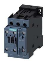
power contactor, AC-3e/AC-3, 12 A, 5.5 kW / 400 V, 3-pole, 24 V DC, auxiliary contacts: 1 NO + 1 NC, screw terminal, communication-capable
