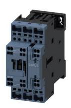
power contactor, AC-3e/AC-3, 12 A, 5.5 kW / 400 V, 3-pole, 24 V AC, 50 Hz, auxiliary contacts: 1 NO + 1 NC, spring-loaded terminal, upright mounting position
