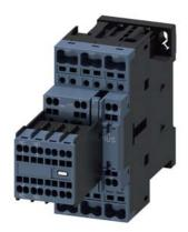
power contactor, AC-3e/AC-3, 12 A, 5.5 kW / 400 V, 3-pole, 24 V AC, 50 Hz, auxiliary contacts: 2 NO + 2 NC, spring-loaded terminal, removable auxiliary switch
